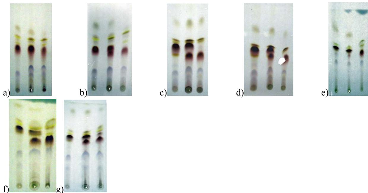
**Figure S1.** TLC images from CuAAC reactions with crude **28** and azides **10** (a), **9** (b), **7** (c), **8** (d), **3** (e), **4** (f), and **5** (g): lane A = crude **2**; lane B = cospot; lane C = reaction mixture at ten minutes. The plates show complete conversion of **2** to triazole products.
