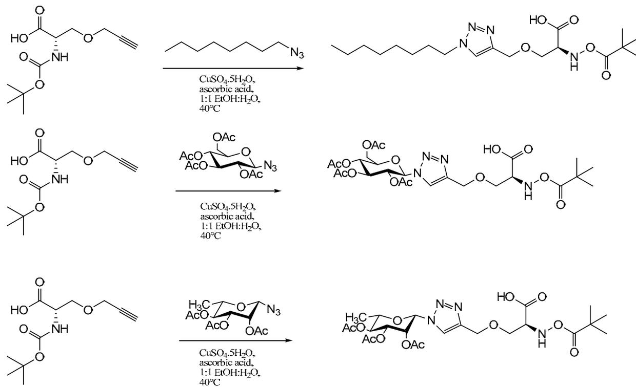
**Scheme S2.** Control CuAAC reactions carried out using alkyne **1** and azides **3**, **5** and **8**.
