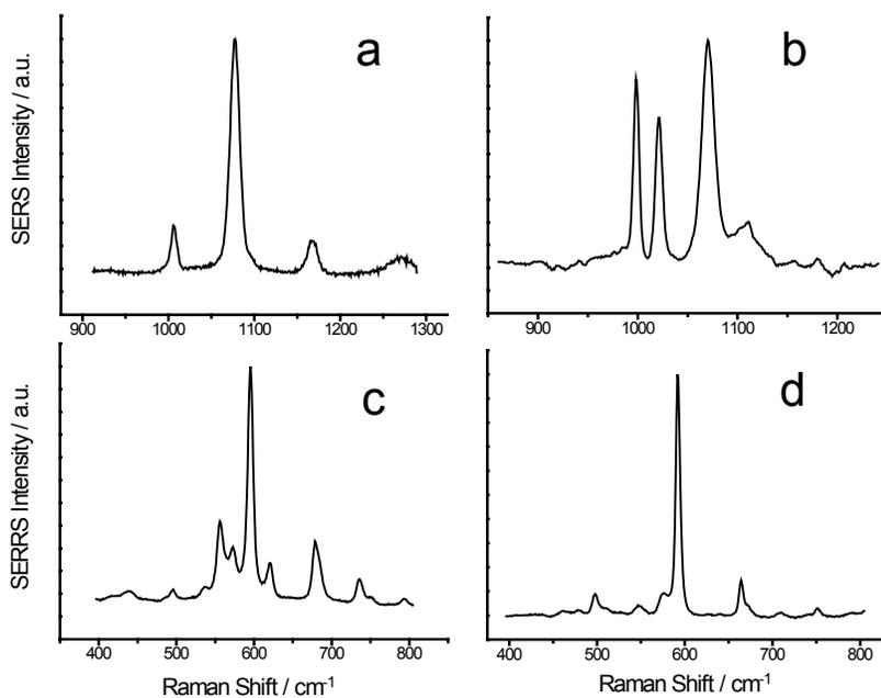
**Figure S3.** SERS spectra of the probe molecules. a, HTP; b, TP; c, Ox; d, NBA.
