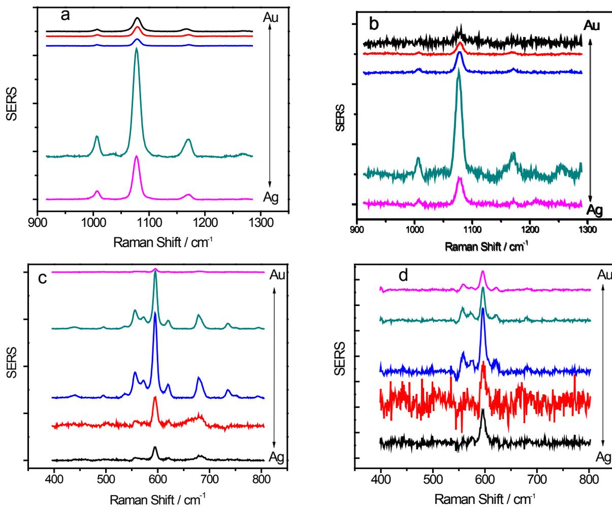
**Figure S4:** SERS spectra of HTP (a and b) Oxazine (c and d) and on the NPs at different 632.8 nm (a and c) and 785 nm (b and d). In all the figures, from top to bottom, pure Au, 9Au:1Ag, 5Au:5Ag, 1Au:9Ag, and pure Ag.
