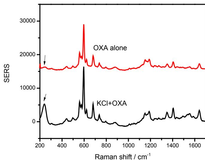
**Figure S5:** Effect of excess halide (0.1 M KCl was added to the colloid before drying) on the SERRS intensity (sample composition: Au<sub>9</sub>:Ag<sub>1</sub>). Notice that no strong Metal – halide stretching vibration (indicated by an arrow) was observed when the colloid was dried only in the presence of OXA. However, that band is significant when KCl was added. The SERRS signal in the presence of KCl was consistently stronger than in the absence of excess Cl<sup>-</sup>.
