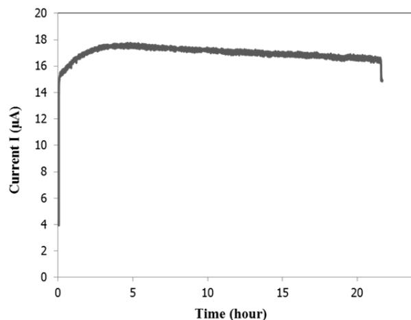
**Fig. S3.** Current over 24 h under illumination, by PEDOT-1/ITO-PET in seawater, at an applied potential of +0.70 V (vs. Ag/AgCl; Pt counter electrode).
