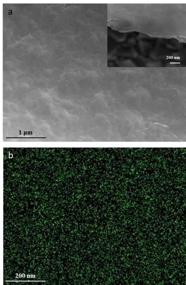
**Fig. S2.** (a) High-Resolution Scanning Electron Micrograph (HRSEM) of PEDOT-1 thin film, and (b) EDX-ray mapping image of Mn in PEDOT-1 in the same area.
