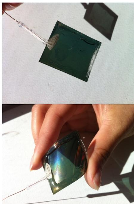
**Fig. S1.** Digital images of the as-prepared flexible electrode comprising PEDOT-1 thin film deposited onto ITO-coated PET.
