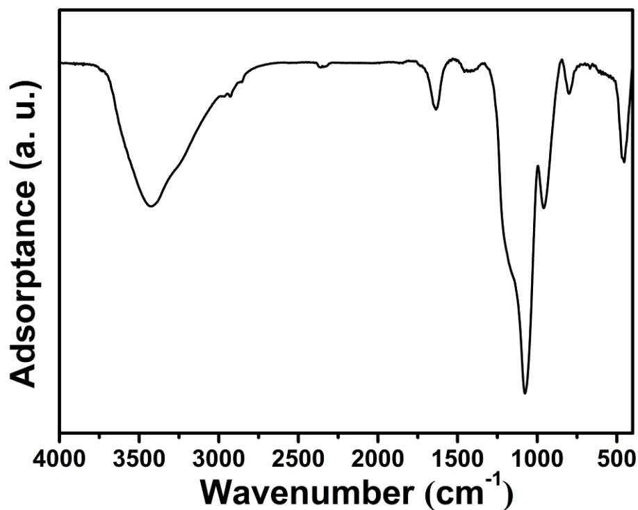
**Fig. S2** FT-IR spectrum of STPNM-6. The appearance of absorption bonds around 1100, 800, 460 cm<sup>-1</sup> corresponds to Si–O–Si groups.<sup>1</sup> The peak around 935 cm<sup>-1</sup> is attributed to the Ti–O–Si bonds and the band at 400-600 cm<sup>-1</sup> indicates the presence of the Ti–O–Ti bonds.<sup>2</sup> The wide peak bond at 3424 cm<sup>-1</sup> proves the presence of –OH.<sup>3,4</sup>
