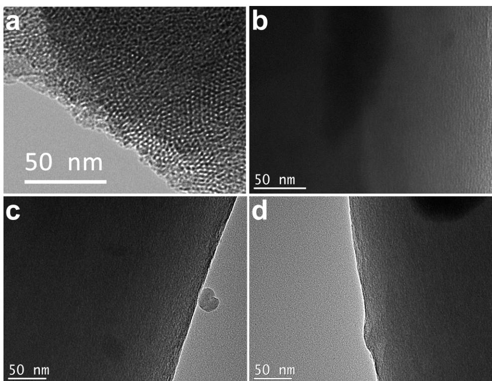
**Fig. S4** TEM images of pure silica nanofibrous membrane (a) and STPNMs with Si/Ti molar ratio of 24, 18 and 12 (b-d), respectively.
