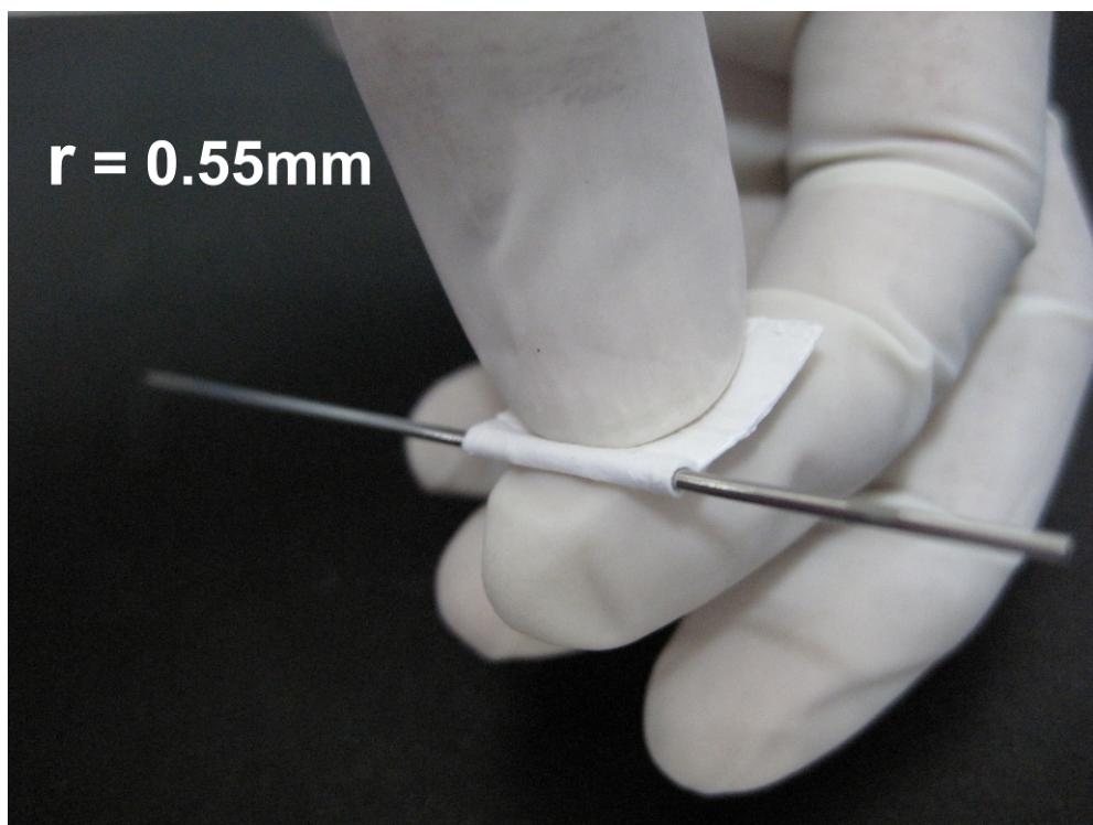
**Fig. S1** STPNM-6 curved to 0.55 mm radius of curvature.
