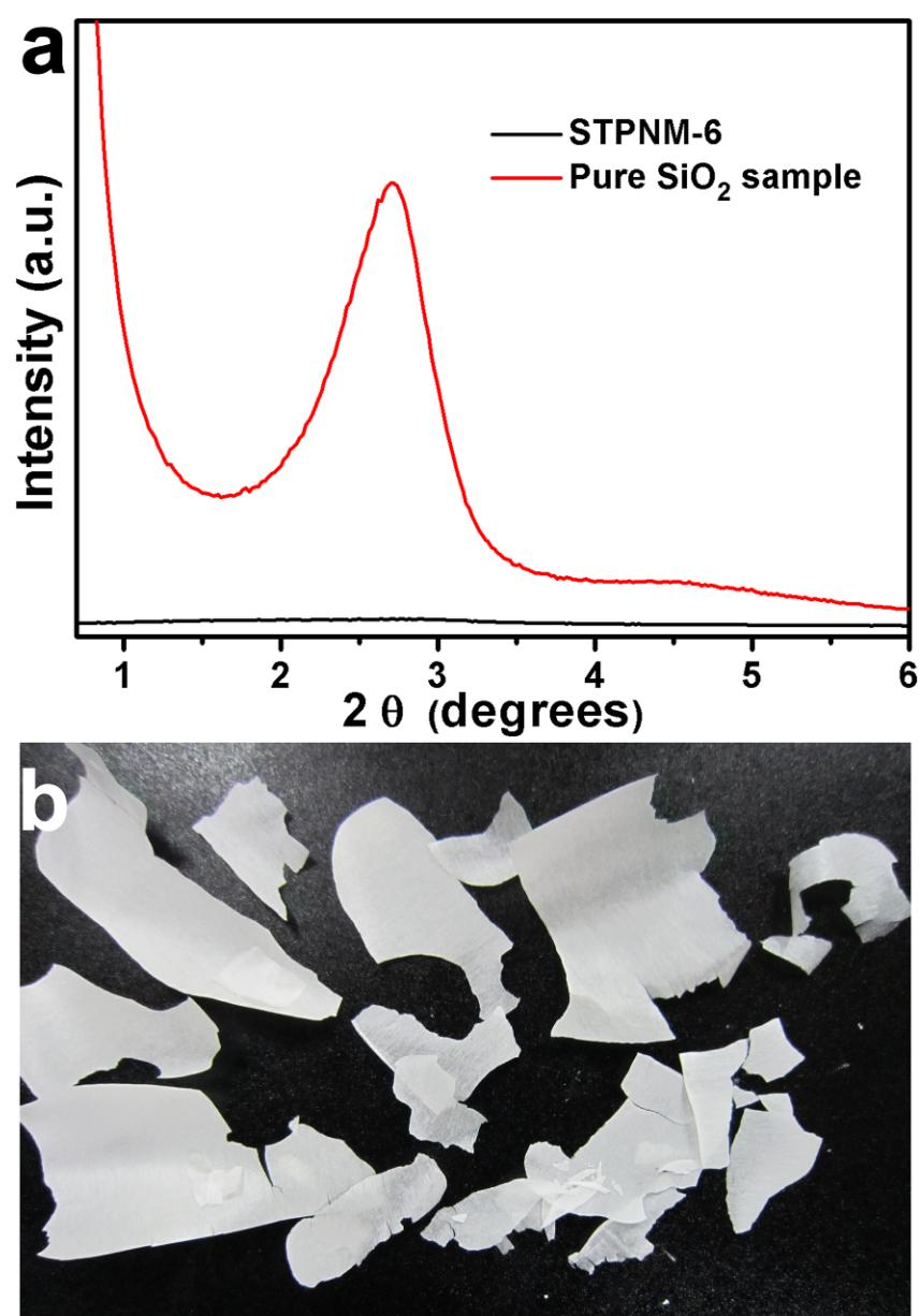
**Fig. S3** (a) Small-angle XRD patterns of pure silica nanofibrous membrane (black) and STPNM-6 (red), respectively. (b) Optical images of pure silica nanofibrous membrane after calcination.
