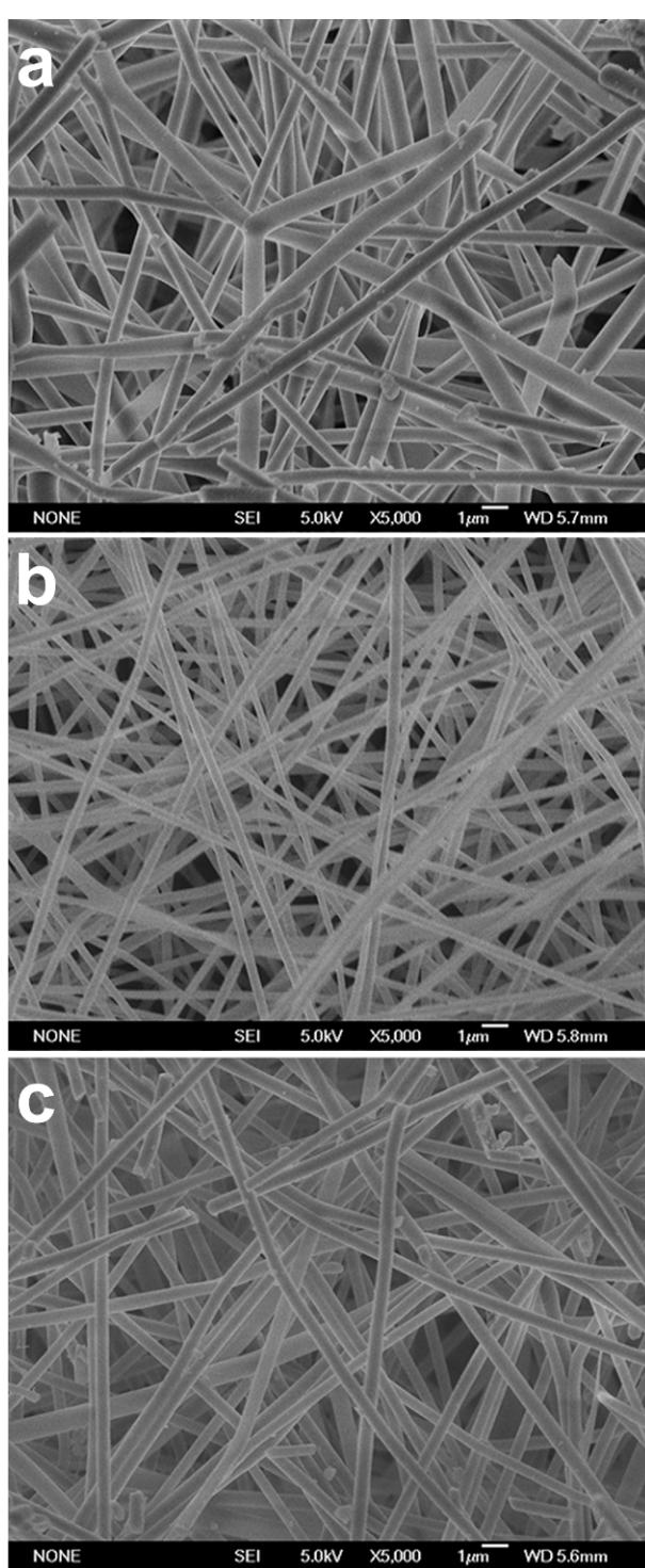
**Fig. S5** SEM images of STPNMs with Si/Ti molar ratio of 24, 18 and 12 (a-c), respectively.
