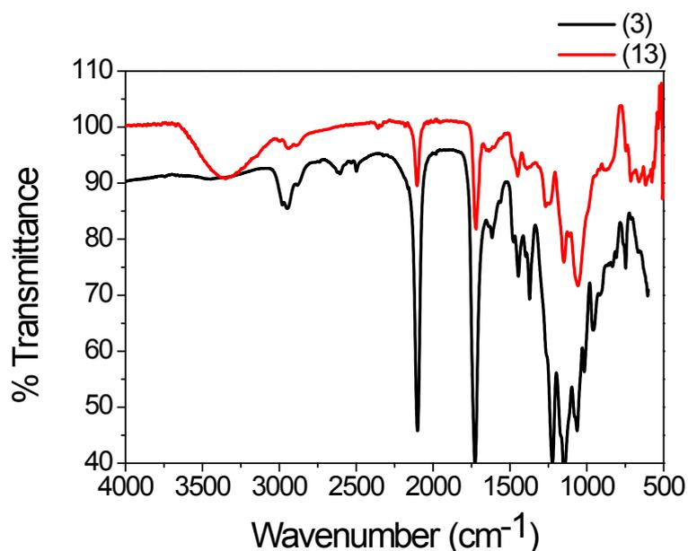
**Figure S16.** Infrared spectra of azide-functional polymer **(3)** and following 1,3-dipolar cycloaddition reaction with  $\beta$ -D-1-propargyl galactose **(13)**.
