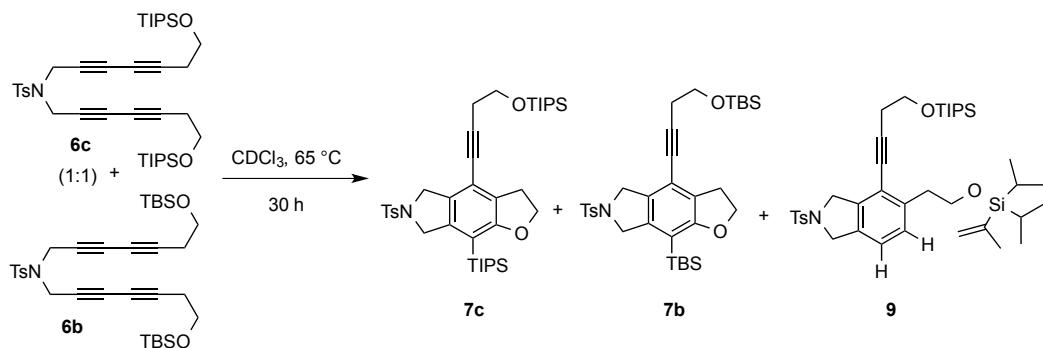
A nearly equimolar solution of tetracynes **6b** (12 mg, 0.02 mmol) and **6c** (14 mg, 0.02 mmol) in chloroform-*d* (1 mL) was kept at  $65^\circ\text{C}$ . Reaction progress was followed by  $^1\text{H-NMR}$  and LCMS. After 32 h only products **7b** and **7c** were observed; there was no evidence for the presence of cross-over products **7d** and **7d'**, whose presence would have been detected by both  $^1\text{H-NMR}$  and LCMS analysis.
