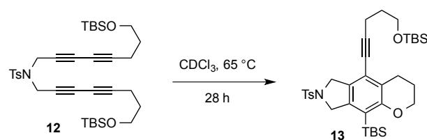
A solution of tetrayne **12** (7 mg, 0.011 mmol) in chloroform-*d* (0.6 mL, 0.018 M) was kept at 65 °C for 28 h. Reaction was monitored by  $^1\text{H-NMR}$  spectral analysis. Once the approximate reaction rate was known, the following experiment was performed on a scale suitable for isolation and characterization of product **13**.
