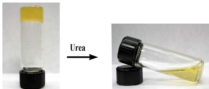
**Figure S1.** Photograph of gel-sol transition upon addition of urea (concentration of **1** was 2 wt%).
