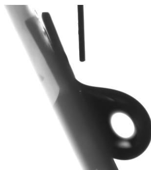
ESI. 3 The image of 20μL water droplet sticking on the tilted PU film. the title angle is 66°
