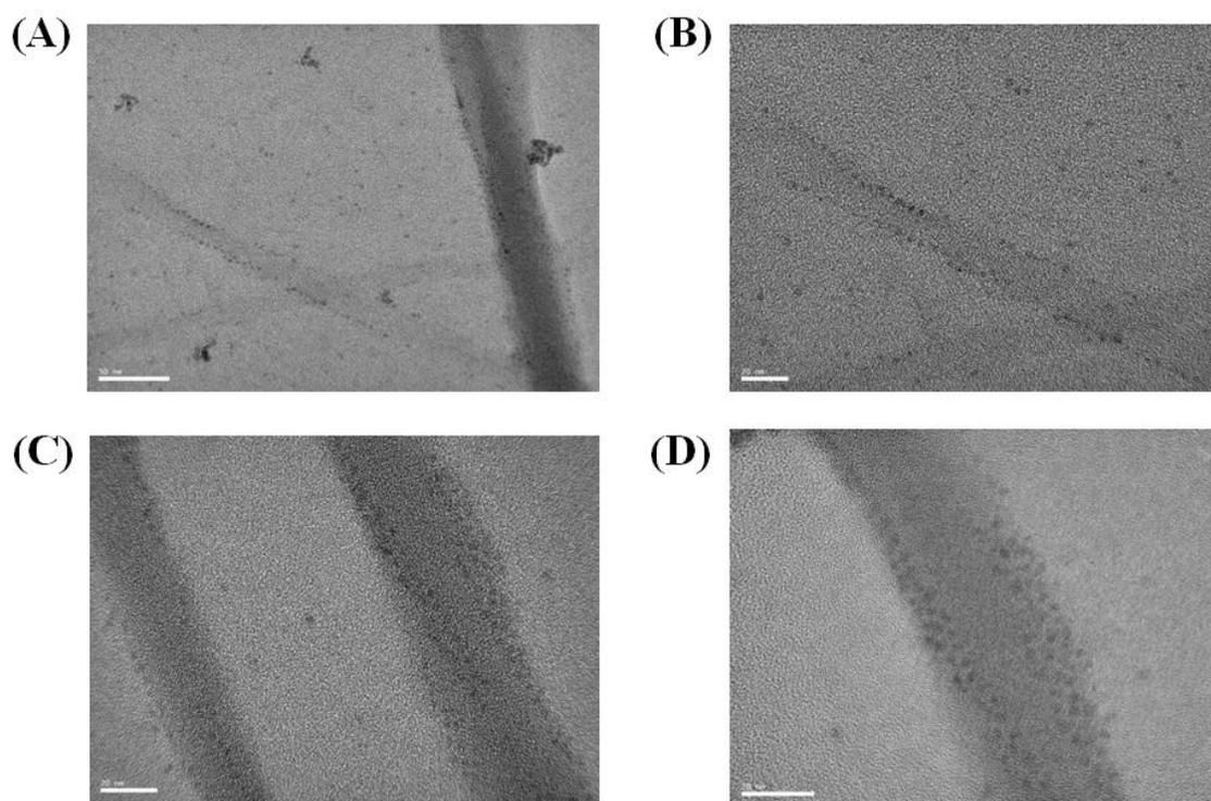
Figure S1. TEM micrographs of the fibrillar structure of the cyclophane **1** xerogel containing CdSe/ZnS QDs.
