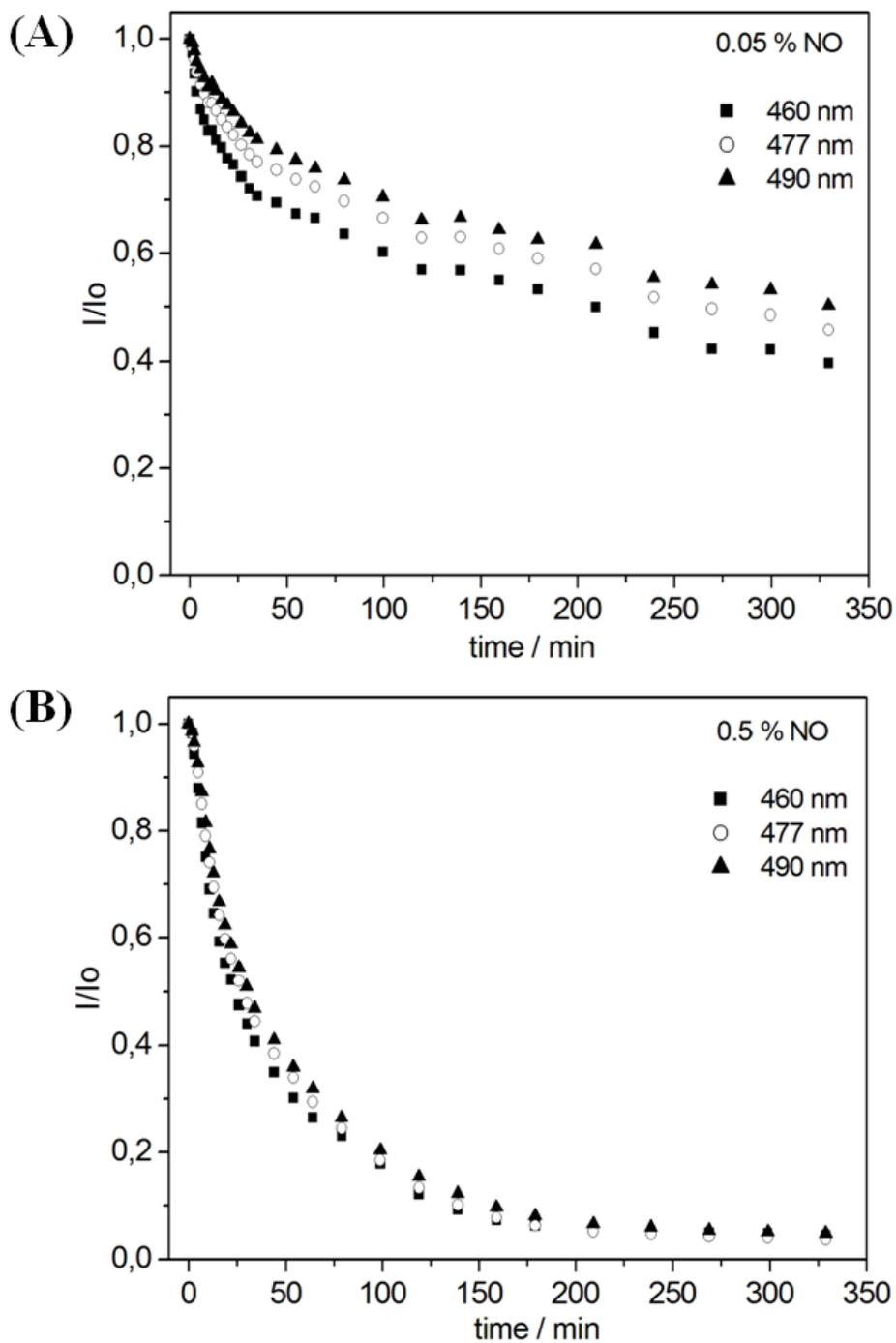
Figure S6. Evolution along the time of the fluorescence intensity at different emission wavelengths (460 nm, 477 nm and 490 nm) of the QDs (0.45  $\mu$ M) in the toluene organogel of cyclophane **1** (2.6 mg/mL) in the presence of different concentrations of NO: A) 0.05 % NO, B) 0.5 % NO.
