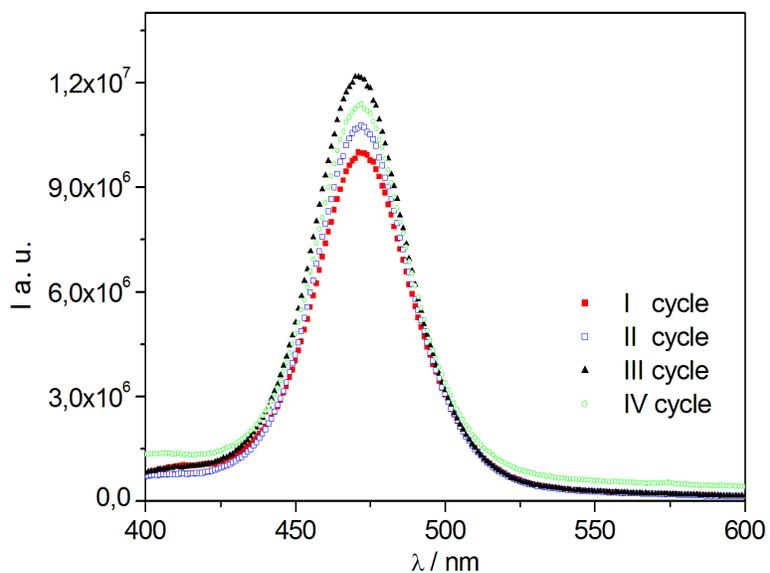
Figure S3. Emission spectra of samples prepared in toluene containing CdSe/ZnS QDs ( $0.75 \mu\text{M}$ ) and organogelator **1** ( $2.7 \text{ mg/mL}$ ) ( $\lambda_{\text{exc}} = 366 \text{ nm}$ ). The organogels were heated to achieve a clear solution, followed by cooling to room temperature to reform the gel. The cycle was repeated four times in the same cuvette and the emission spectra of the samples were measured 30 minutes after formation of the organogel.
