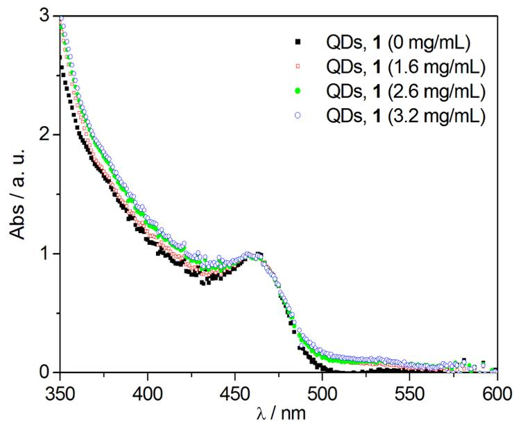
Figure S2. Absorption spectra of samples prepared in toluene containing CdSe/ZnS QDs ( $0.45 \mu\text{M}$ ) and different concentrations of organogelator **1**. The absorption spectra have been corrected at 600 nm and normalized at 457 nm to allow comparison of the shape and position of the absorption maxima.
