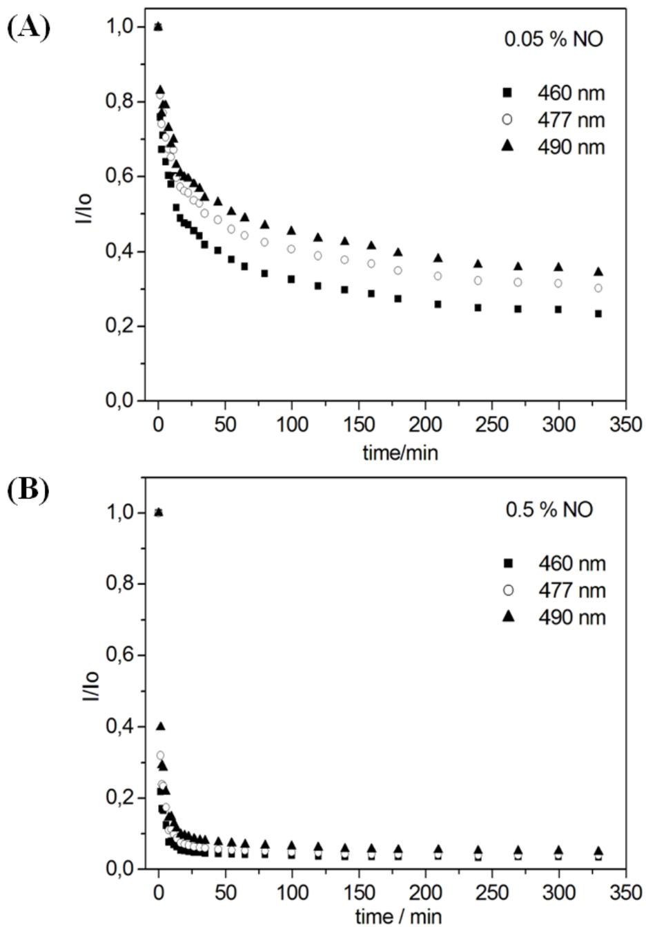
Figure S7. Evolution along the time of the fluorescence intensity at different emission wavelengths (460 nm, 477 nm and 490 nm) of the QDs ( $0.45 \mu\text{M}$ ) in toluene in the presence of different concentrations of NO: A) 0.05 % NO, B) 0.5 % NO.
