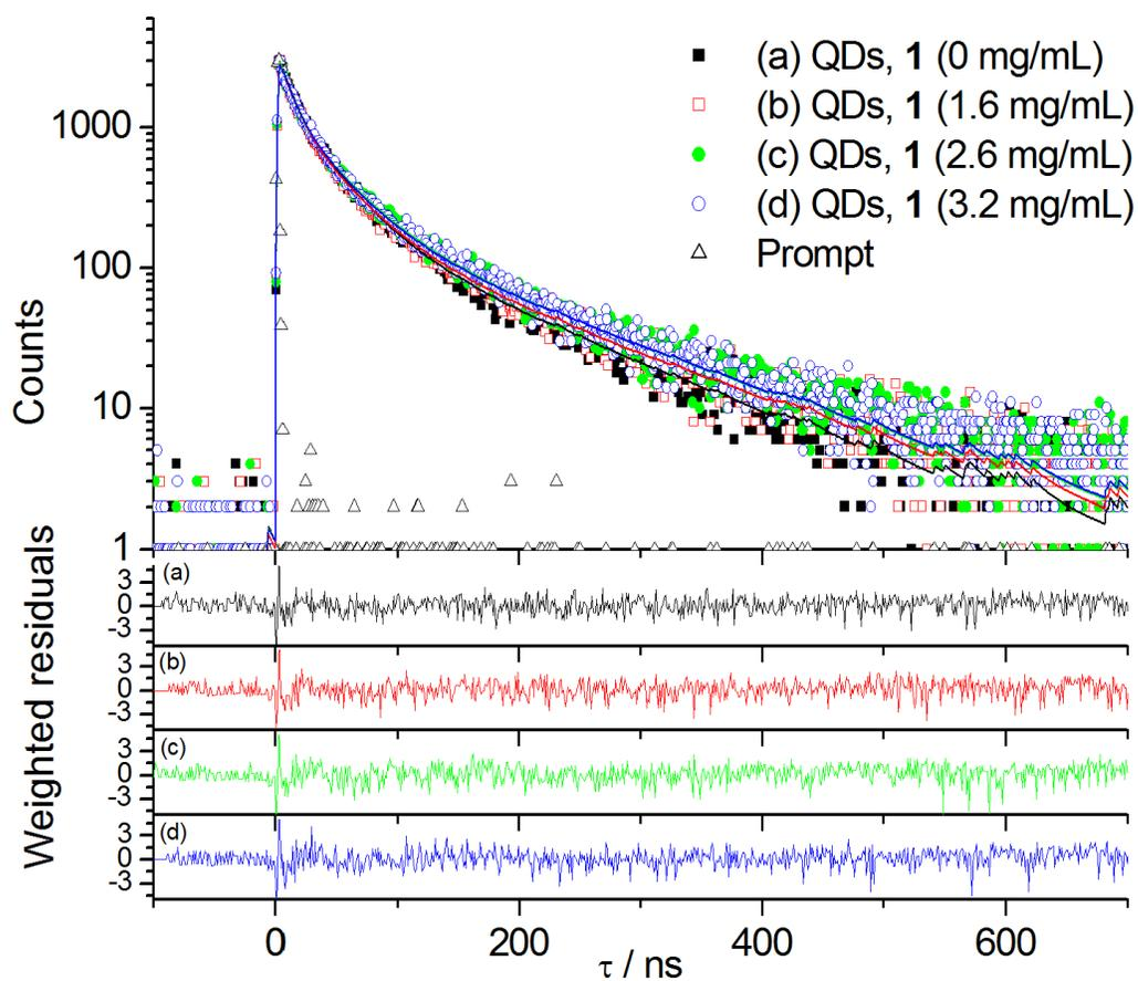
Figure S4. Fluorescence decay traces and weighted residuals of CdSe/ZnS QDs (0.45 μM) in toluene and toluene organogel containing different concentrations cyclophane **1** ( $\lambda_{\text{exc}} = 372$  nm,  $\lambda_{\text{em}} = 480$  nm). The incident light pulse is also shown (open triangles).
