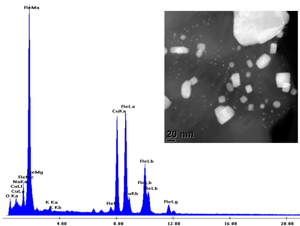
**Figure S1.** EDX analysis of a region of supported large crystals. The Cu signal comes from the holey carbon grid on which the material was deposited for imaging.
