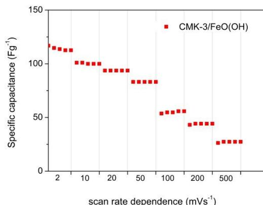
**Fig. ESI-1** Potential scan rate dependence of the iron (hydr)oxide CMK-3 nanocomposite. (The integral specific capacitance of the electroactive material is shown for each of the five cycles at each potential scan rate.)
