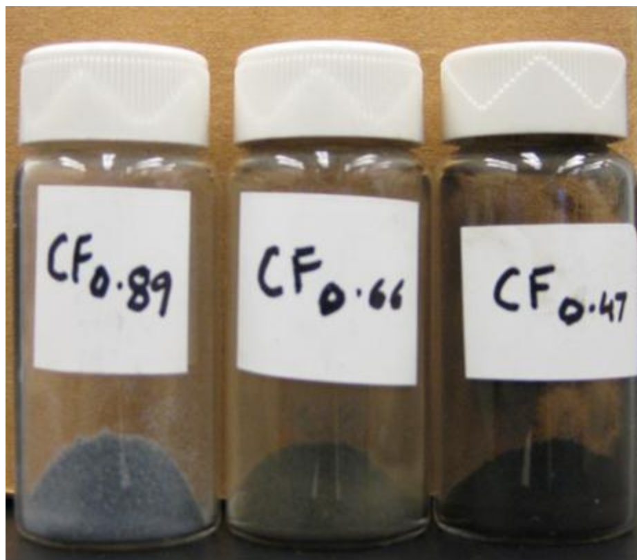
Figure S2: Picture indicating the color darkening with decreased fluorine content for fluorinated graphene.
