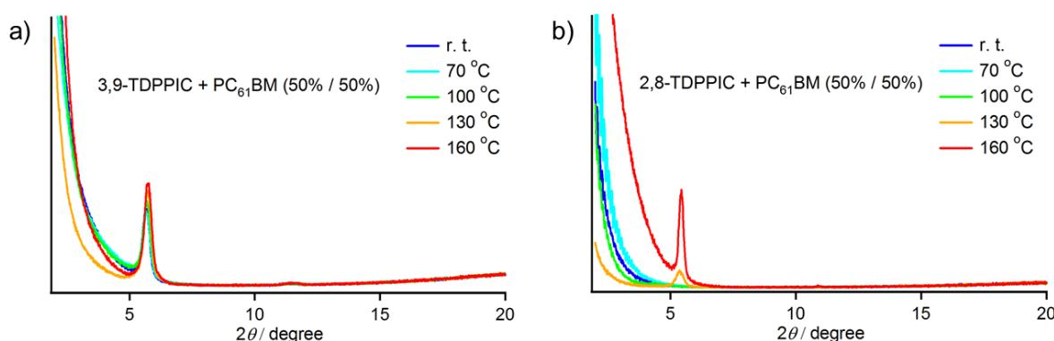
**Fig. S1** XRD diffraction patterns of thin films of a) 3,9-TDPPIC:PCBM (5:5) and b) 2,8-TDPPIC:PCBM (5:5). The diffraction patterns of thermally annealed films with various annealing temperatures (as-cast, 70, 100, 130, and 160 °C) are also shown by color curves. The films were prepared by drop-cast of their chloroform solutions onto glass substrate.
