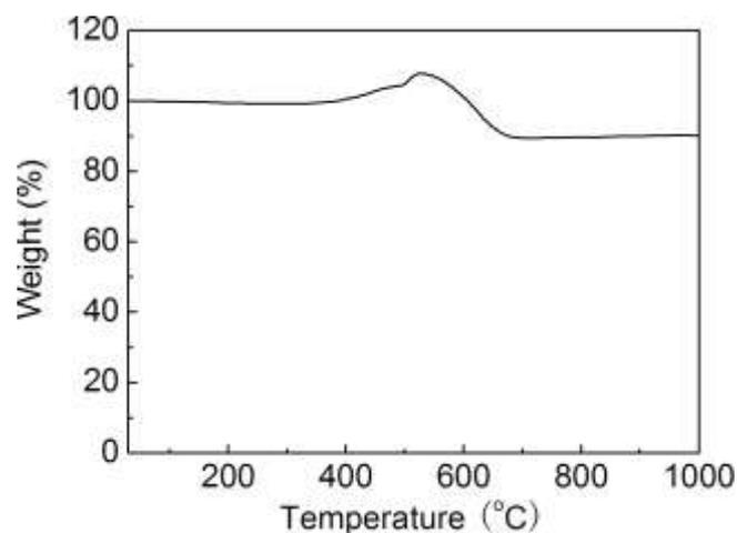
**Figure S4.** TG analysis curves of SbNP/MWCNT under air atmosphere at a heating rate of  $10\text{ °C min}^{-1}$ .
