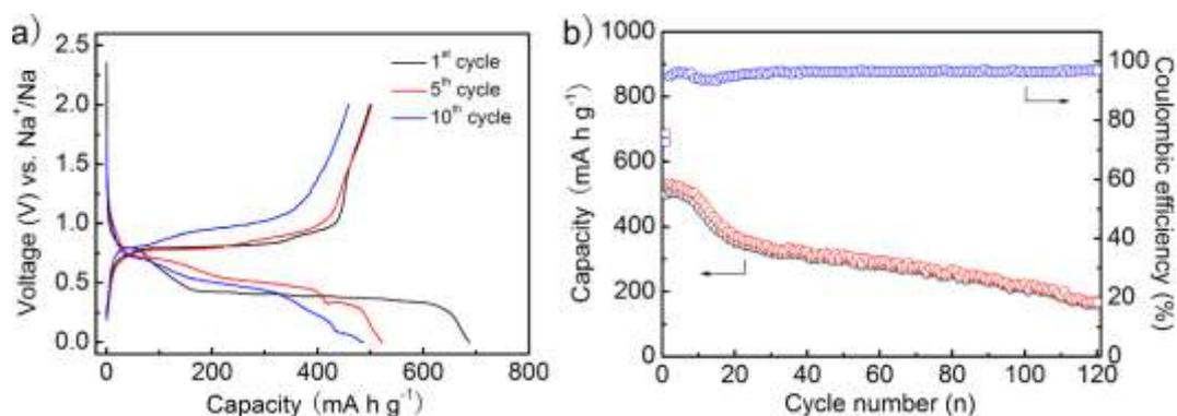
**Figure S9.** a) Galvanostatic charge/discharge profiles and b) cycling performance and Coulombic efficiency of the SbNP/MWCNT electrode in the voltage range of 0 to 2 V vs. Na<sup>+</sup>/Na using 1 M NaClO<sub>4</sub> in EC/PC with addition of 10% FEC as the electrolyte. The first ten cycles are under 0.1 A g<sup>-1</sup> and the remaining cycles are under 0.2 A g<sup>-1</sup>.
