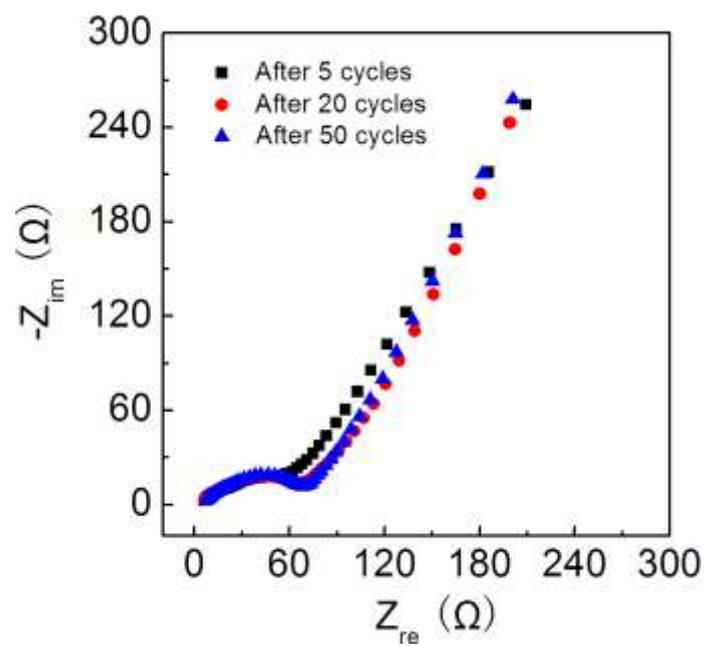
**Figure S11.** Nyquist plots of the SbNP/MWCNT electrode for different cycles.
