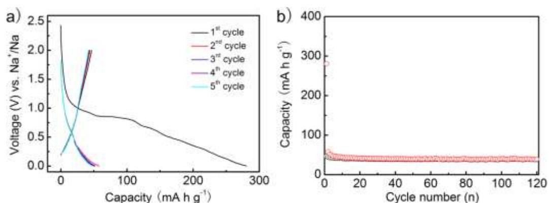
**Figure S8.** a) Galvanostatic charge/discharge profiles and b) cycling performance of the MWCNT electrode in the voltage range of 0 to 2 V vs. Na<sup>+</sup>/Na. The first ten cycles are under 0.1 A g<sup>-1</sup> and the remaining cycles are under 0.2 A g<sup>-1</sup>.
