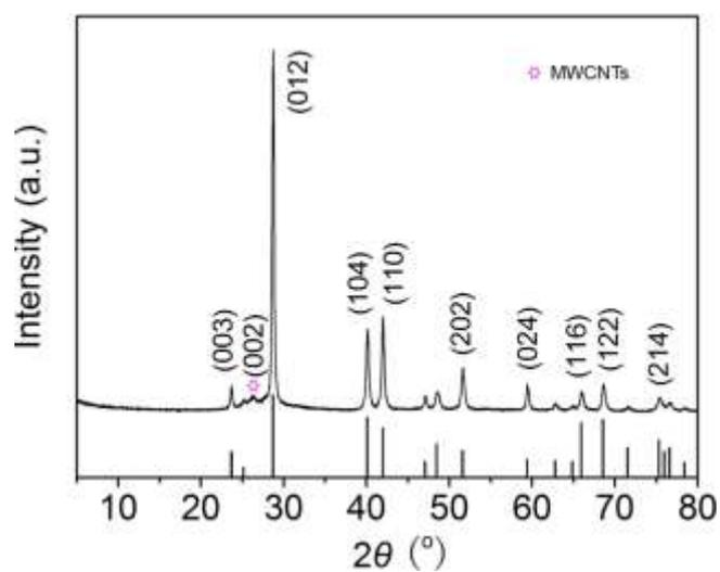
**Figure S2.** XRD pattern of SbNP/MWCNT. The peak marked with a red asterisk corresponds to the (002) plane of MWCNTs.
