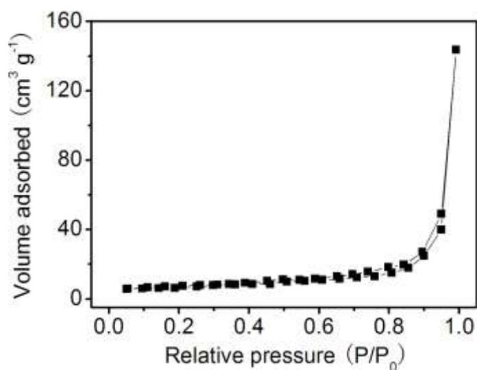
**Figure S3.** Nitrogen adsorption/desorption isotherms of SbNP/MWCNT.
