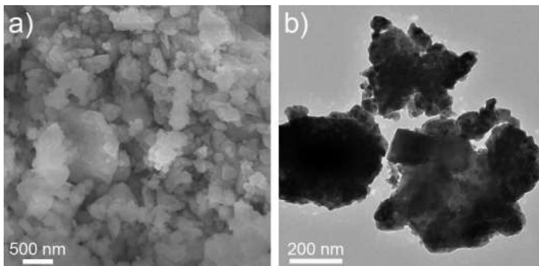
**Figure S5.** (a) SEM and (b) TEM images of wet milled Sb powder.
