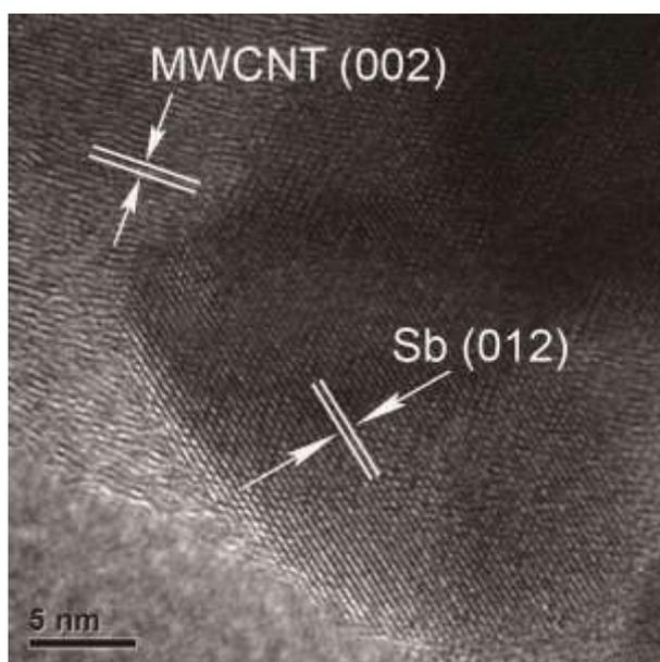
**Figure S10.** HRTEM of the SbNP/MWCNT electrode after 120 cycles.
