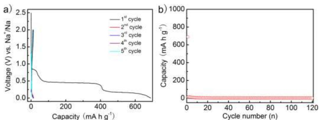
**Figure S7.** a) Galvanostatic charge/discharge profiles and b) cycling performance of the Sb electrode in the voltage range of 0 to 2 V vs. Na<sup>+</sup>/Na. The first ten cycles are under 0.1 A g<sup>-1</sup> and the remaining cycles are under 0.2 A g<sup>-1</sup>.
