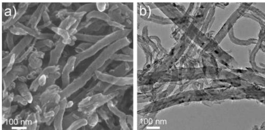
**Figure S6.** (a) SEM and (b) TEM images of wet milled MWCNTs.
