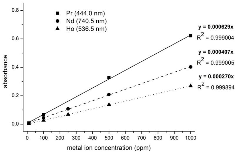
Figure S2: Calibration curves for  $\text{Pr}^{3+}$  (444.0 nm),  $\text{Nd}^{3+}$  (740.5 nm) and  $\text{Ho}^{3+}$  (536.5 nm).
