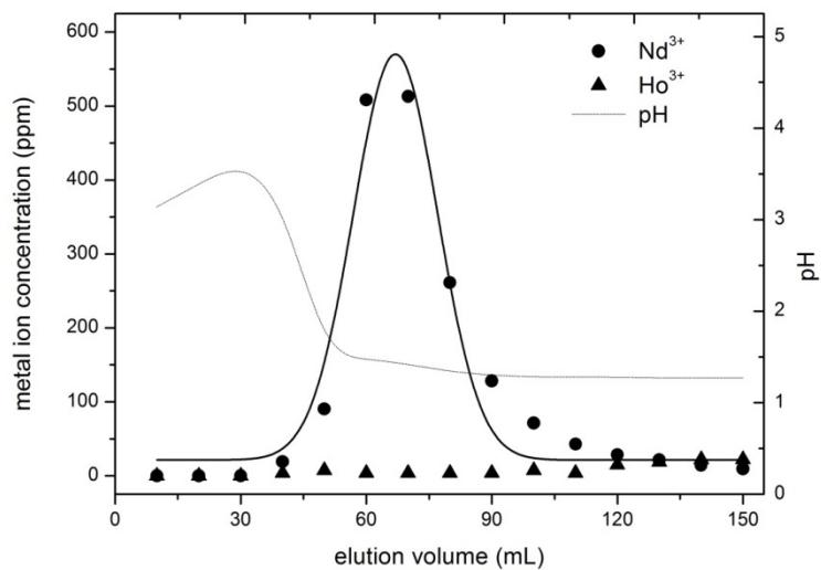
Figure S9: Breakthrough curve Nd<sup>3+</sup>/Ho<sup>3+</sup> separation (excess Nd<sup>3+</sup>) with DTPA-chitosan/silica at pH 1.25.
