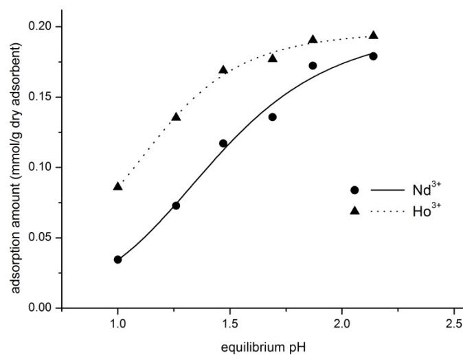
Figure S6: Selective adsorption amount for EDTA-chitosan as a function of equilibrium pH.
