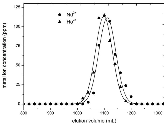
Figure S7: Chromatogram of  $\text{Nd}^{3+}/\text{Ho}^{3+}$  separation (ratio 1:1) with Chelex® 100 at pH 2.
