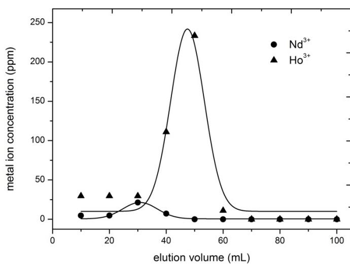
Figure S8: Elution curve for Nd<sup>3+</sup>/Ho<sup>3+</sup> separation (1:1 ratio) with DTPA-chitosan/silica at pH 1.25.
