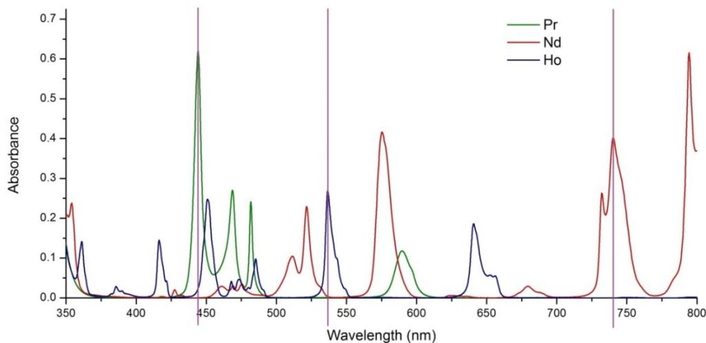
Figure S1: Optical absorption spectra of aqueous solutions (1000 ppm) of  $\text{Pr}^{3+}$ ,  $\text{Nd}^{3+}$  and  $\text{Ho}^{3+}$ . The following wavelengths were used for determining the concentrations of the lanthanides:  $\text{Pr}^{3+}$  (444.0 nm),  $\text{Nd}^{3+}$  (740.5 nm) and  $\text{Ho}^{3+}$  (536.5 nm). These wavelengths are indicated by vertical lines in the spectra.
