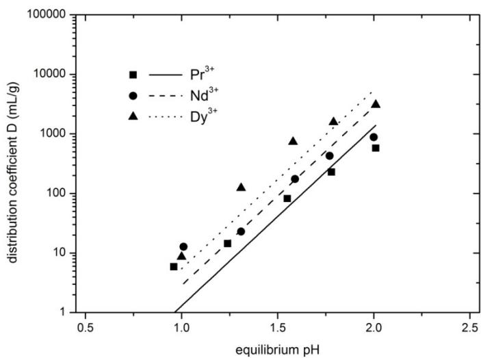
Figure S5: EDTA-chitosan distribution coefficient for some lanthanide ions as a function of equilibrium pH. The data points are linearly fitted with a fixed slope of 3.
