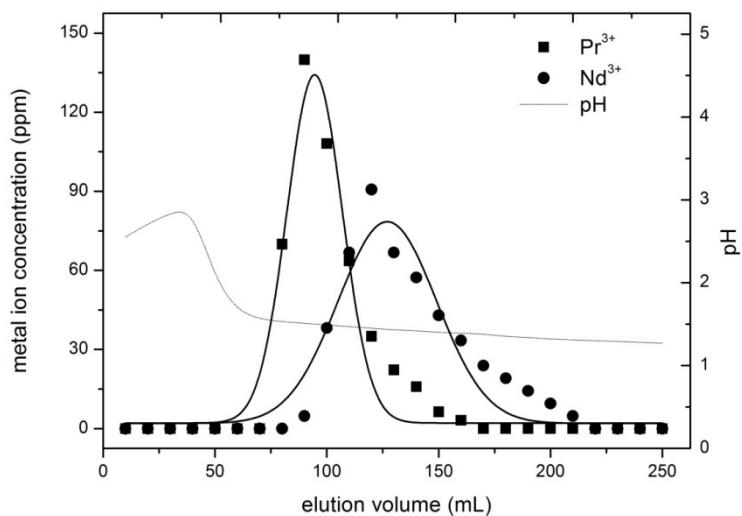
Figure S11: Chromatogram of Pr<sup>3+</sup>/Nd<sup>3+</sup> separation (1:1 ratio) with DTPA-chitosan at pH 1.50.
