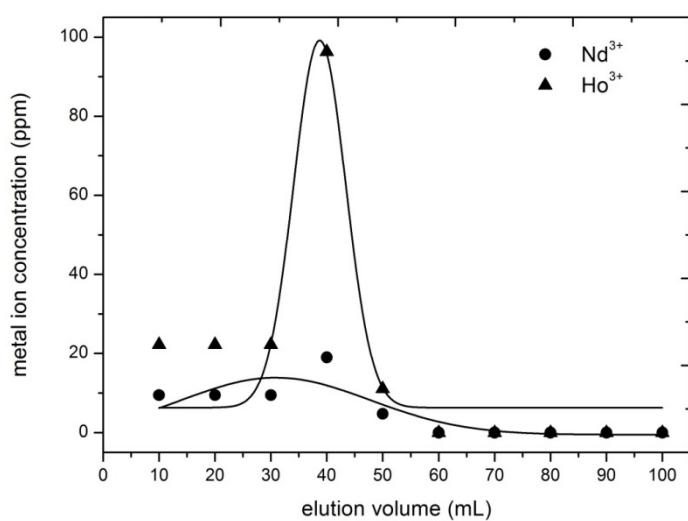
Figure S10: Elution curve Nd<sup>3+</sup>/Ho<sup>3+</sup> separation (excess Nd<sup>3+</sup>) with DTPA-chitosan/silica.
