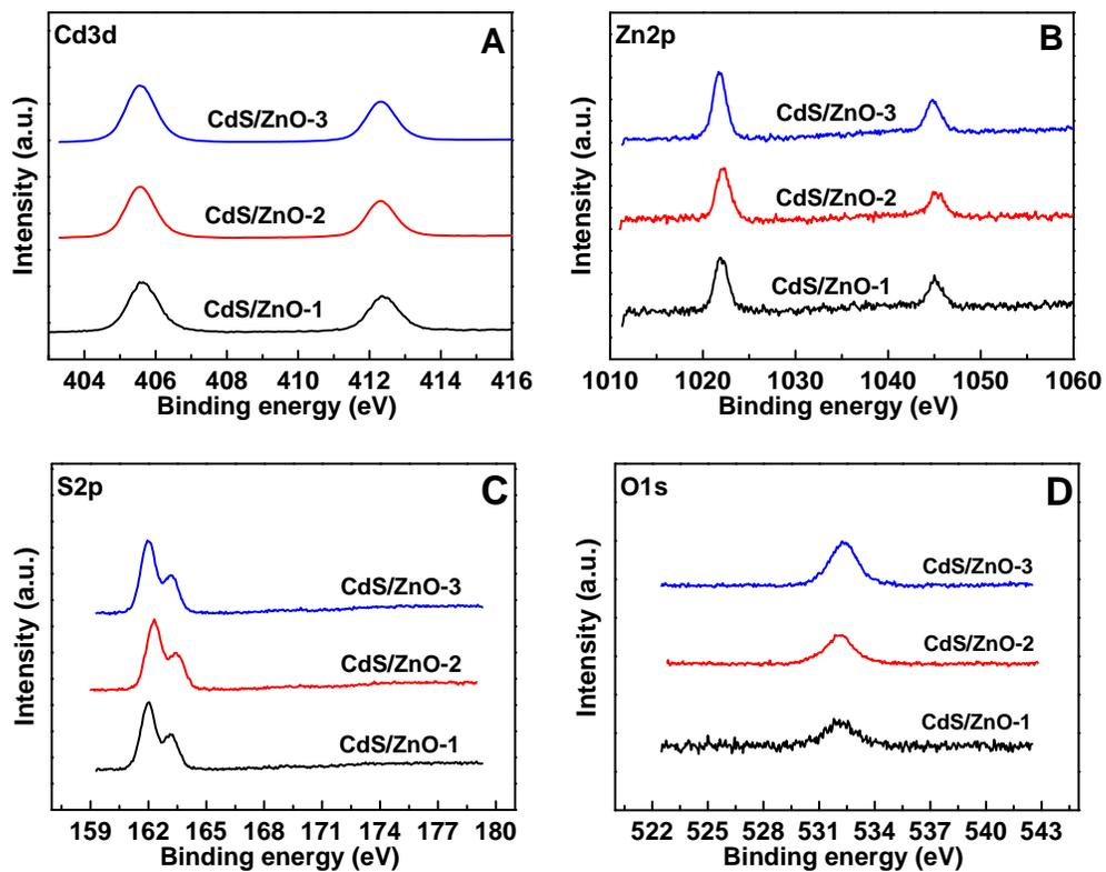
**Figure S7.** High-resolution XPS spectra of (A) Cd3d, (B) Zn2p, (C) S2p, and (D) O1s for the CdS/ZnO nanocomposite materials.
