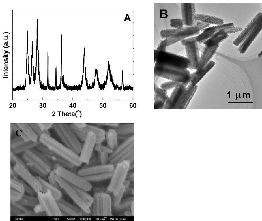
**Figure S11.** (A) XRD pattern (B) TEM image and (C) SEM image of CdS/ZnO-1 after photocatalytic reaction.
