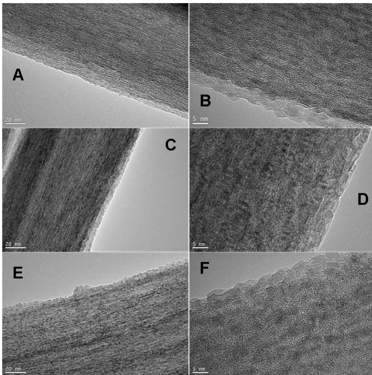
**Figure S4.** TEM and HRTEM images of (A,B) ZnS/CHA-1, (C,D) ZnS/CHA-2 and (E,F) ZnS/CHA-3.
