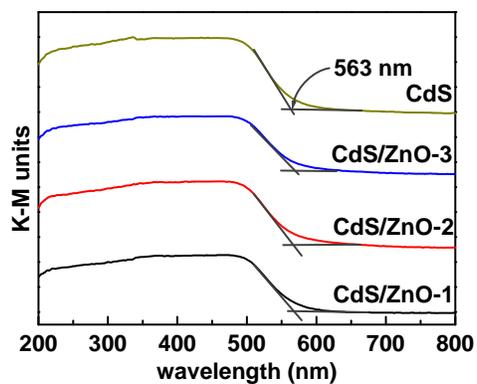
**Figure S10.** UV/Vis diffuse reflectance spectra of CdS/ZnO-1, CdS/ZnO-2, CdS/ZnO-3 and pure CdS.
