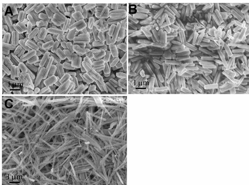
**Figure S1.** SEM images of (A) ZnS/CHA-1, (B) ZnS/CHA-2, and (C) ZnS/CHA-3.
