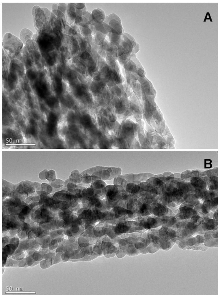
**Figure S9.** TEM images of (A) CdS/ZnO-1 and (B) CdS/ZnO-2.
