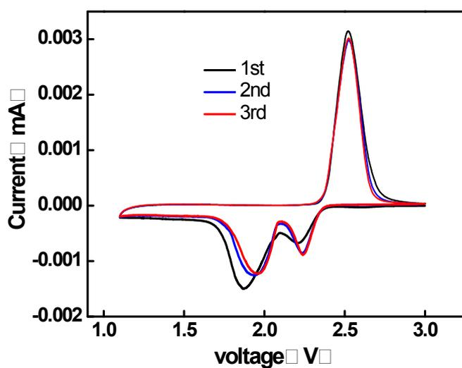
**Fig. S7** The first three CV curves of CTF-1/S@155°C composite electrode.
