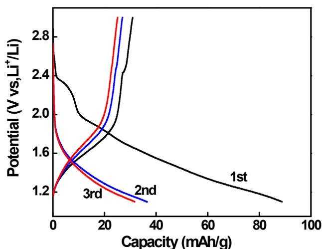
**Fig. S6** The discharge and charge curves of the CTF-1 substrate at a current density of 30 mA/g in 1 M LiTFSI/DOL-DME electrolyte.
