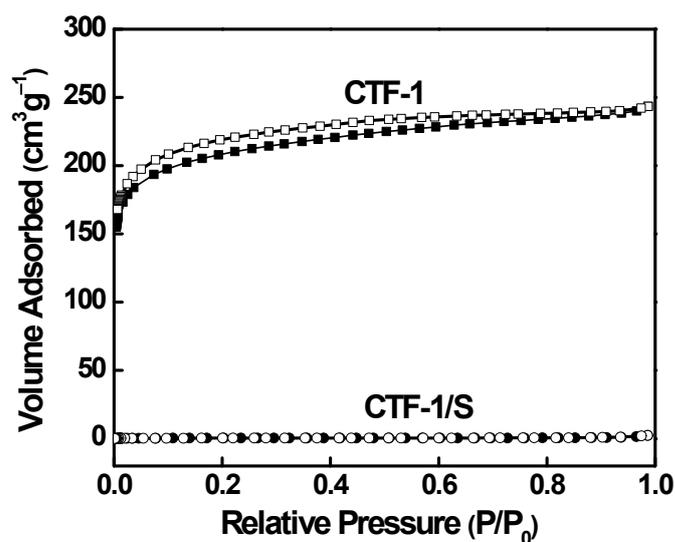
Fig. S2 N<sub>2</sub> adsorption/desorption isotherms before and after impregnation with sulfur.
