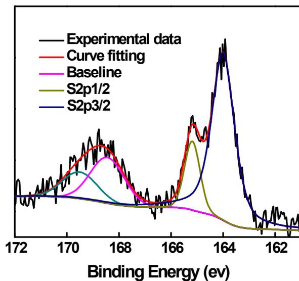
**Fig. S4** XPS S2p spectra of sulfur powder.
