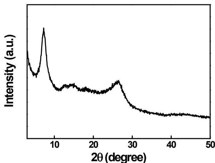
**Fig. S1** The XRD spectrum of CTF-1/S@155°C composite after removing the sulfur ( $\lambda = 1.54056 \text{ \AA}$ ).
