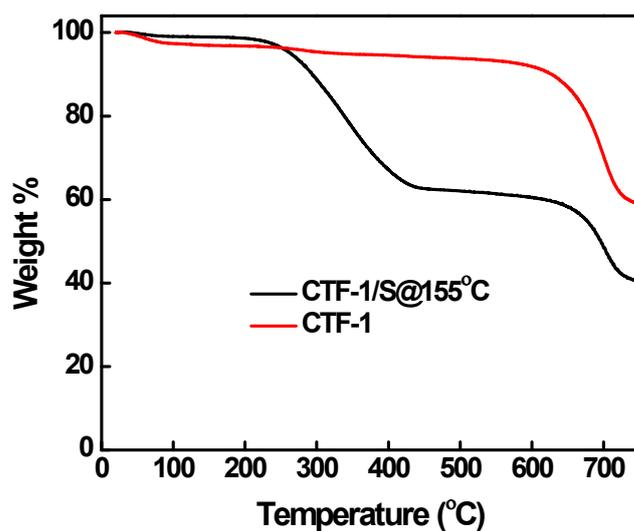
**Fig. S5** TGA curves of CTF-1 and CTF-1/S@155°C composite recorded in N<sub>2</sub> atmosphere.
