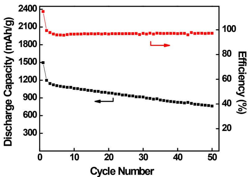
**Fig. S8** Cycling performance of the CTF-1/S@155 °C composites at a rate of 0.1 C current density in 1 M LiTFSI/DOL-DME electrolyte.
