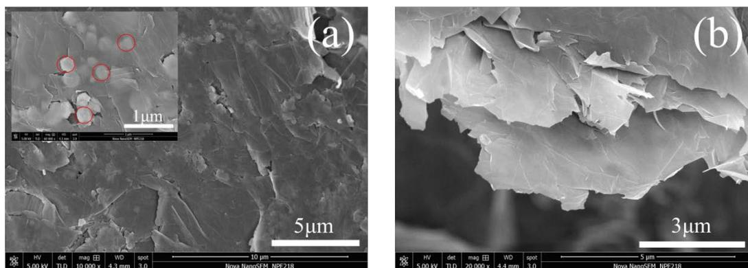
Figure S3. (a) SEM images of the prepared GNNM electrode. The details are shown in the inset image; (b) SEM image for the side view of GNNM electrode.
