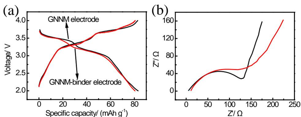
Figure S5. (a) The first galvanostatic charge–discharge profiles of GNNM electrode and GNNM-binder electrode; (b) The Nyquist plots of GNNM electrode and GNNM-binder electrode charged/discharged after 3 cycles.
