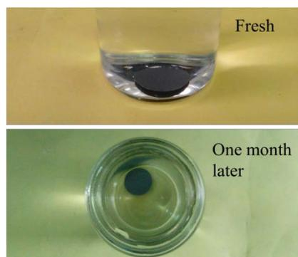
Figure S4. Photos of GNNM electrode for fresh and stored in the 1.0 M NaClO<sub>4</sub>/EC+PC (1:1, v/v) electrolyte one month.
