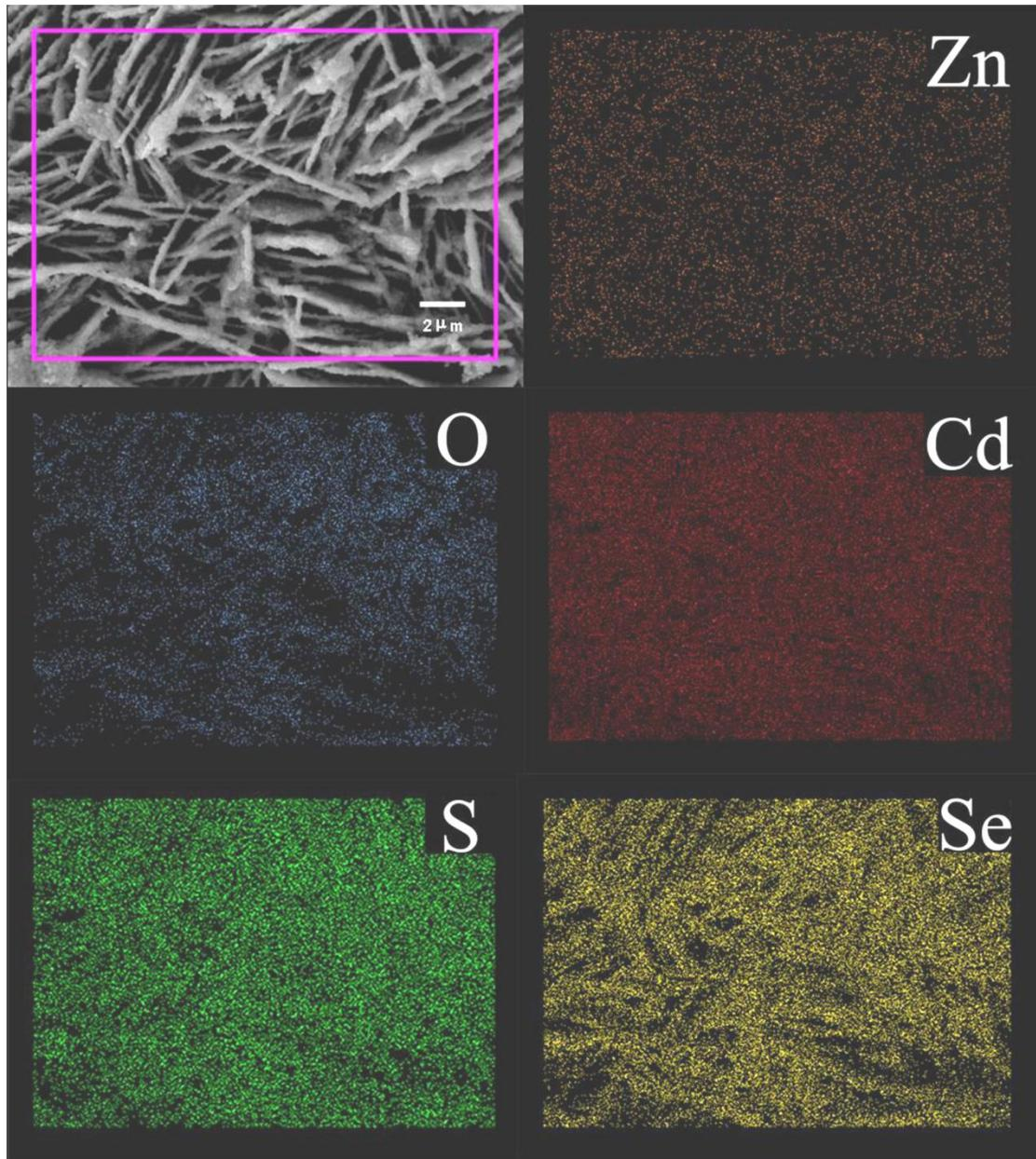
**Figure S2.** SEM image of CdSe/CdS/ZnO nanostructures and energy-dispersive X-ray spectroscopy (EDS) mapping images of zinc (Zn), oxygen (O), cadmium (Cd), sulfur (S) and selenium (Se), respectively.
