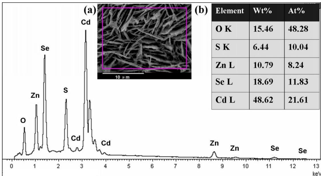
**Figure S3.** EDS spectrum of the CdSe/CdS/ZnO nanostructures with inserted (a) SEM images and (b) chemical composition table.
