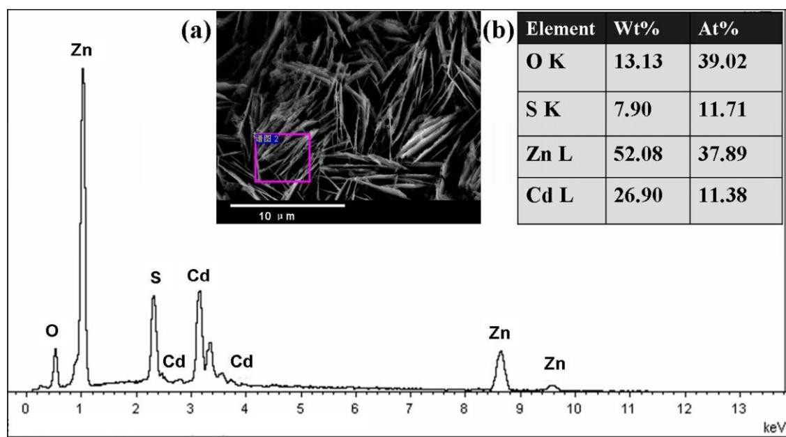
**Figure S1.** EDS spectrum of the CdS/ZnO nanostructure with inserted (a) SEM images and (b) chemical composition table.
