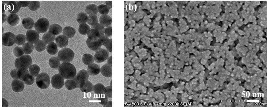
**Fig. S2** (a) TEM image of the Au nanoparticle showing its size ranges from 8 nm to 14 nm. (b) SEM image showing that Au particles are rejected by the SWCNT/PD composite film rather than adsorb onto the film.
