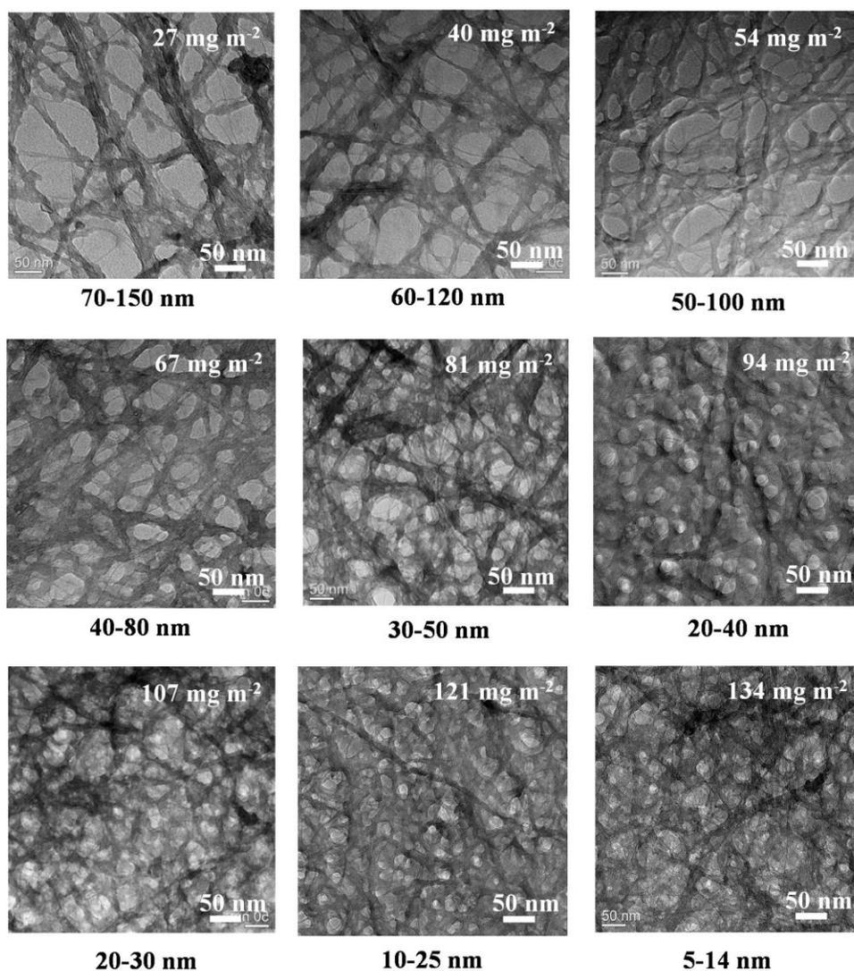
**Fig. S1** TEM images and pore size of SWCNT/PD composite films with usage of SWCNT/PD of  $27 \text{ mg m}^{-2}$ ,  $40 \text{ mg m}^{-2}$ ,  $54 \text{ mg m}^{-2}$ ,  $67 \text{ mg m}^{-2}$ ,  $81 \text{ mg m}^{-2}$ ,  $94 \text{ mg m}^{-2}$ ,  $107 \text{ mg m}^{-2}$ ,  $121 \text{ mg m}^{-2}$  and  $134 \text{ mg m}^{-2}$ , respectively.
