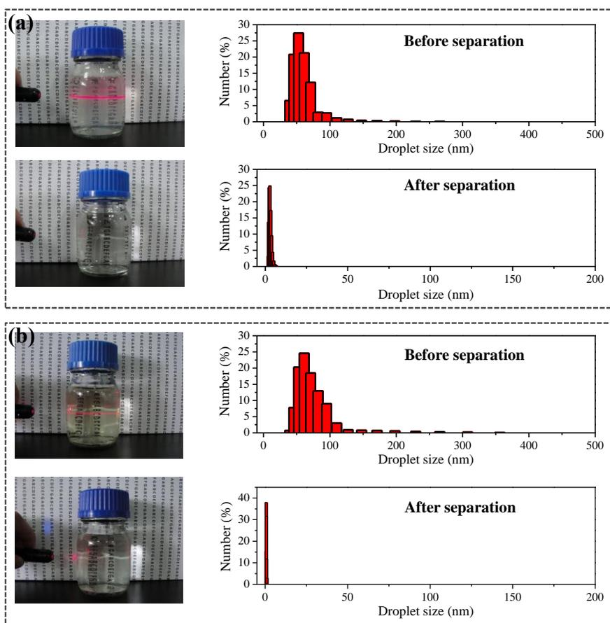
**Fig. S5** Digital photos (left) and oil droplet size distribution (right) of the 1,2-dichloroethane-in-water nanoemulsion (a) and the industrial oil-in-water nanoemulsion (b) before and after separation by a 158-nm-thick SWCNT/PD/PEI composite film.
