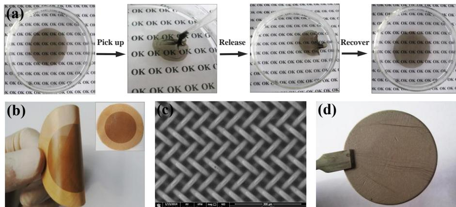
**Fig. S4** (a) A cycle of picking up and releasing a free-standing SWCNT/PD/PEI composite film (thickness: 158 nm) in a water/acetone solution. When a drop of acetone is placed onto the surface of the film, the film spreads out again. Optical image (b) and SEM image (c) of the SWCNT/PD/PEI film transferred onto a copper mesh. (d) Optical image of the SWCNT/PD/PEI film transferred onto a ceramic membrane.
