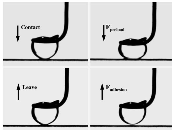
**Fig. S3** Photographs of dynamic underwater oil-adhesion force measurement on the SWCNT/PD/PEI composite film. A 1,2-dichloroethane droplet was used as the detecting probe to contact (upper images) and then leave (lower images) the surface of the film.
