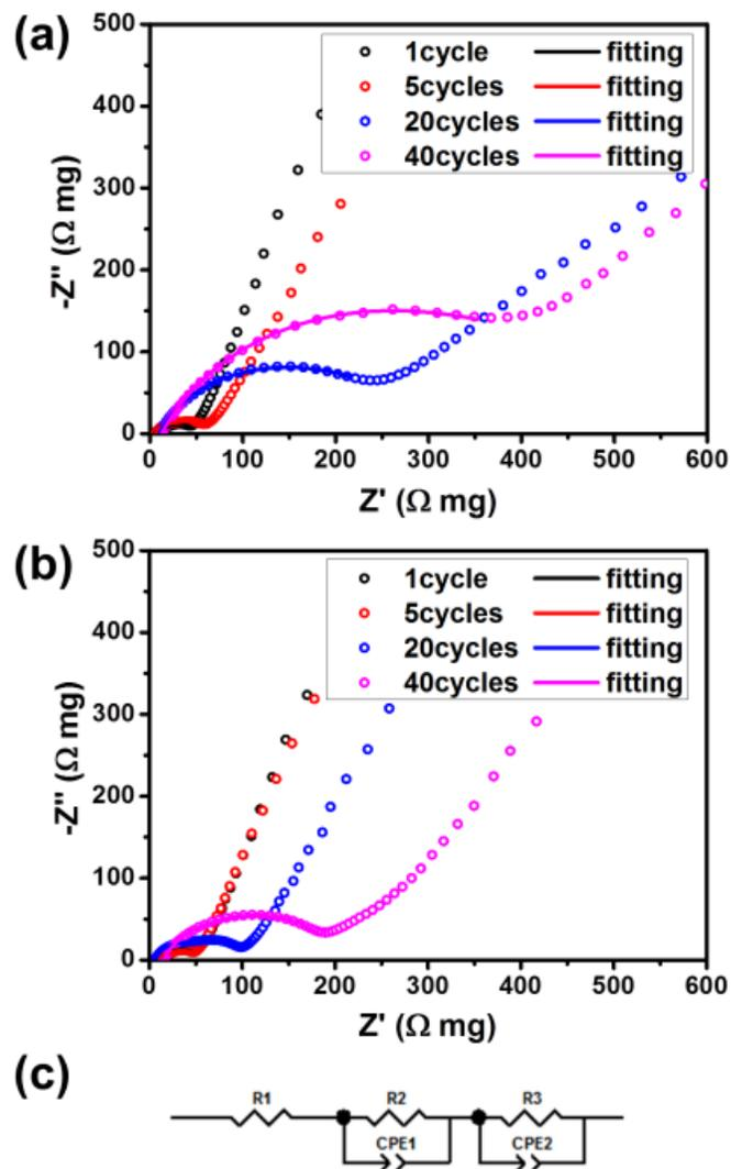
**Fig. S7.** Impedance spectra and curve fitting results for the (a) Si- $\text{Al}_2\text{O}_3$ @C and (b) Si-NiSi<sub>2</sub>- $\text{Al}_2\text{O}_3$ @C composites. (c) Simplified equivalent circuit used for the curve fitting.
