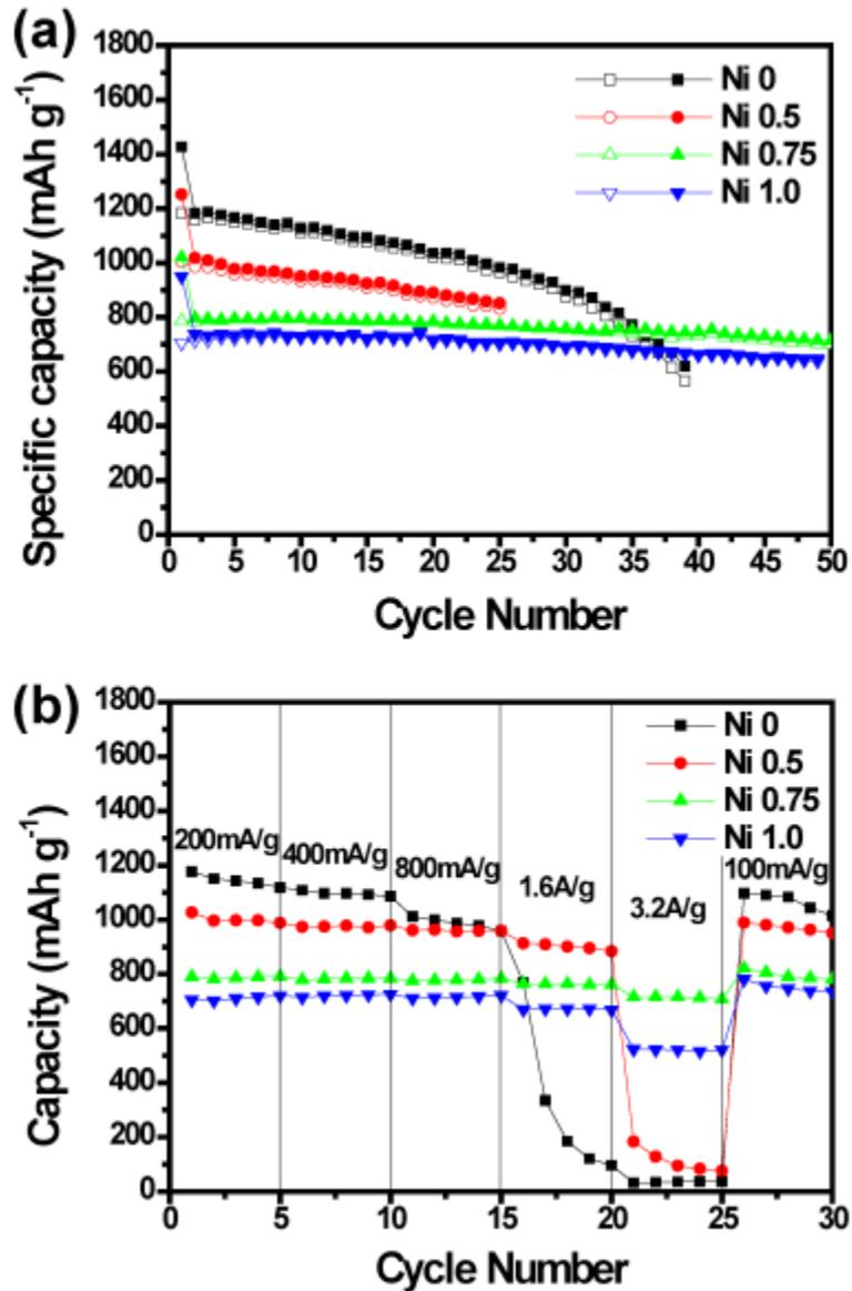
**Fig. S2.** (a) Cycle performance of the Si-Al<sub>2</sub>O<sub>3</sub>@C and Si-NiSi<sub>2</sub>-Al<sub>2</sub>O<sub>3</sub>@C composites at a current density of 100 mA g<sup>-1</sup> within a voltage range of 0.0 – 2.0V (vs. Li / Li<sup>+</sup>). (b) Rate performance of the Si-Al<sub>2</sub>O<sub>3</sub>@C and Si-NiSi<sub>2</sub>-Al<sub>2</sub>O<sub>3</sub>@C composites at various current densities. The discharge current density was fixed at 100 mA g<sup>-1</sup>.
