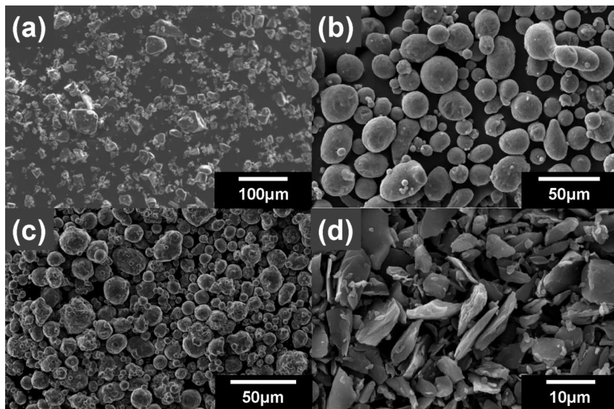
**Fig. S6.** SEM images of the starting materials used for the synthesis of the Si-based composites: (a) SiO, (b) Al, (c) Ni, and (d) graphite.
