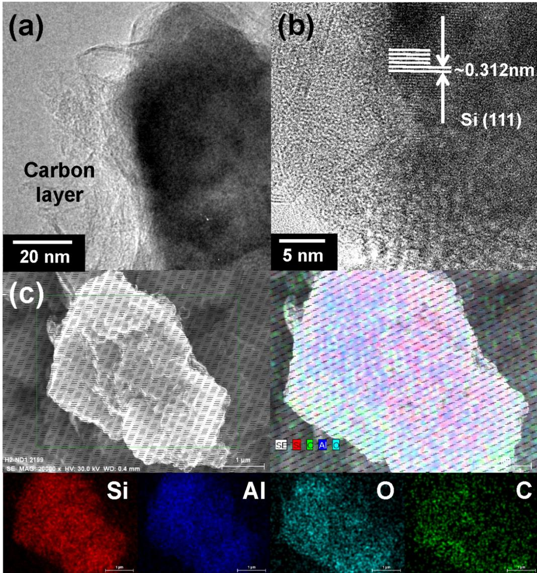
**Fig. S5.** (a) TEM, (b) HRTEM, and (c) STEM images of the Si-Al<sub>2</sub>O<sub>3</sub>@C composite. In the STEM, the corresponding EDS mapping images of each element are also shown with different colors.
