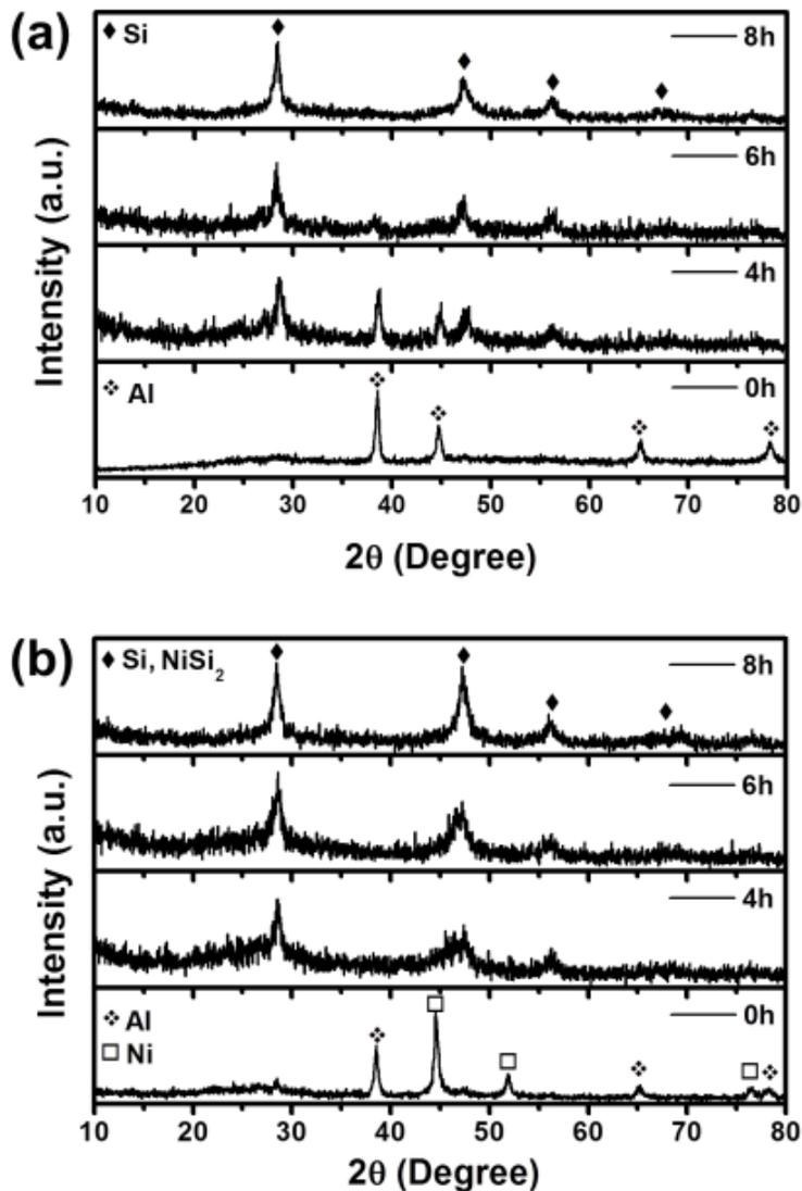
**Fig. S1.** XRD patterns of the (a) Si-Al<sub>2</sub>O<sub>3</sub>@C and (b) Si-NiSi<sub>2</sub>-Al<sub>2</sub>O<sub>3</sub>@C (sample prepared with  $x = 0.75$  in reaction 2) composites after different milling times.
