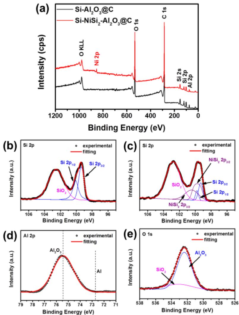
**Fig. S3.** (a) XPS survey spectra of the Si-Al<sub>2</sub>O<sub>3</sub>@C and Si-NiSi<sub>2</sub>-Al<sub>2</sub>O<sub>3</sub>@C composites. XPS peak fitting results of (b) Si 2p spectrum in the Si-Al<sub>2</sub>O<sub>3</sub>@C composite and (c) Si 2p, (d) Al 2p, and (e) O 1s spectra in the Si-NiSi<sub>2</sub>-Al<sub>2</sub>O<sub>3</sub>@C composite.
