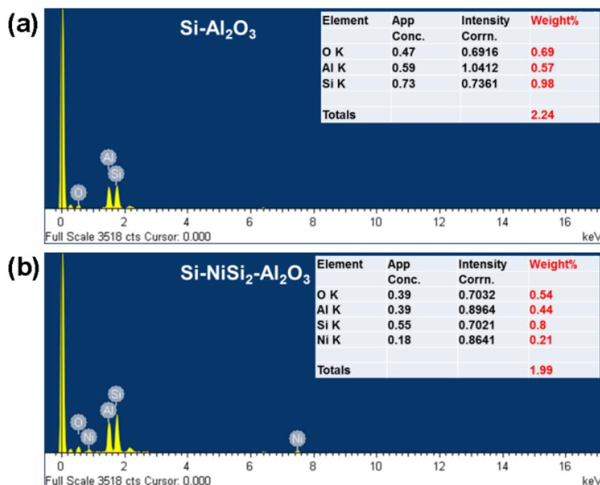
**Fig. S4.** SEM/EDS results of the (a) Si–Al<sub>2</sub>O<sub>3</sub> and (b) Si–NiSi<sub>2</sub>–Al<sub>2</sub>O<sub>3</sub> composites.
