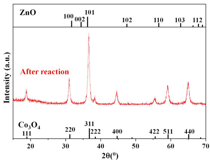
Figure S8. XRD pattern of  $\text{ZnCo}_{1.0}\text{O}_y$  after water oxidation in a reactor – gas chromatography (GC) combination system.
