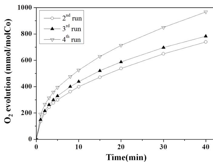
Figure S5. Recycling data of  $\text{ZnCo}_{1.0}\text{O}_y$  in water oxidation using  $\text{Ce(IV)}$  as oxidants.
