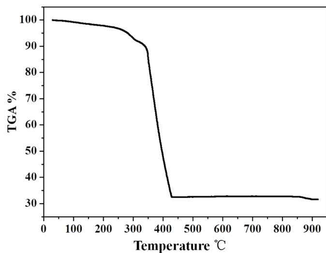
Figure S1. TG profile of Zn-Co<sub>1.0</sub>-coordination polymers.
