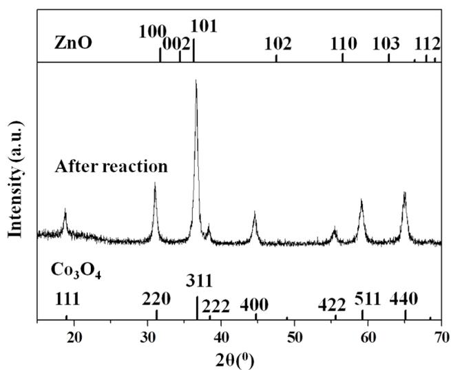
Figure S6. XRD pattern of  $\text{ZnCo}_{1.0}\text{O}_y$  after water oxidation using  $\text{Ce(IV)}$  as oxidant.
