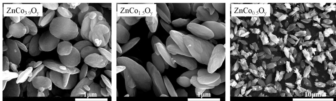
Figure S3. SEM images of a section of ZnCo<sub>x</sub>O<sub>y</sub> oxides.
