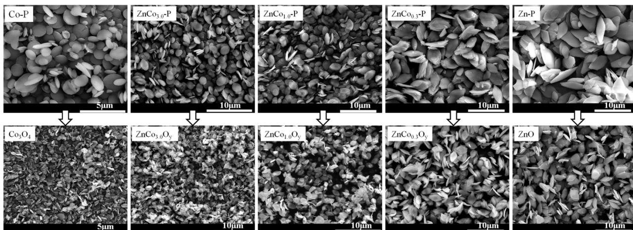
Figure S2. SEM images of a section of Zn-Co<sub>x</sub>-coordination polymer precursors and ZnCo<sub>x</sub>O<sub>y</sub> oxides, the ligand PTCDA was abbreviated as P in the images.
