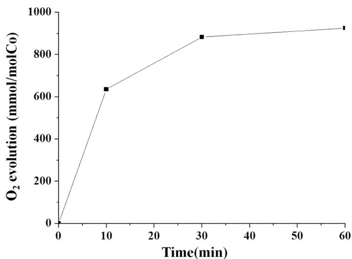
Figure S7. Recycling data of  $\text{ZnCo}_{1.0}\text{O}_y$  in water oxidation utilizing a reactor – gas chromatography (GC) combination system.
