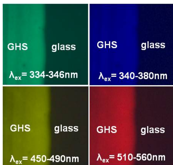
Figure S5. Fluorescent microscopy images of GHS on glass substrate with an excitation wavelength of 334 - 346 nm, 340 - 380 nm, 450 - 490 nm, and 510 - 560 nm.
