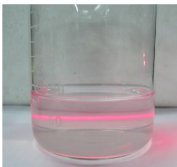
Figure S3 Tyndall effect of Co-Al ELDH colloidal suspension.
