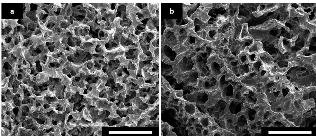
**Fig. S6:** SEM micrographs of cured PGS/PLLA blend scaffolds with a weight ratios of (a) 2.5:1, (b) 3:1 (scale bar: 500  $\mu\text{m}$ ).
