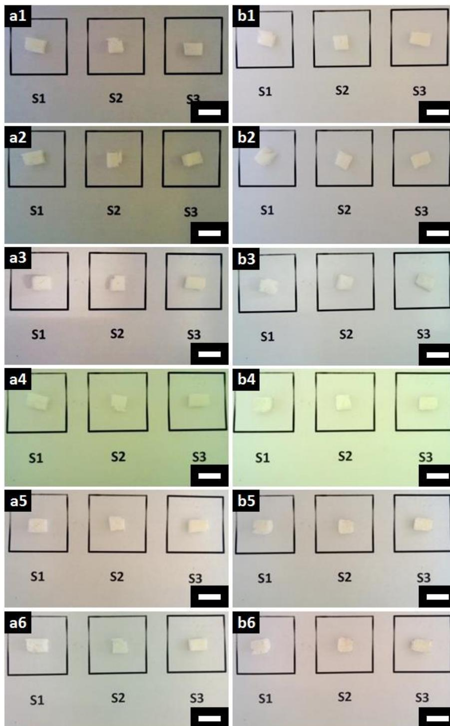
**Fig. S19:** Pictures of PGS/PLLA scaffold samples with a weight ratio of 3:1 during incubation in PBS solution ((a1): Day 0; (a2): Day 1; (a3): Day 7, (a4): Day 15; (a5): Day 23; (a6): Day: 31), and in PBS solution with the addition of lipase enzyme ((b1): Day 0; (b2): Day 1; (b3): Day 7, (b4): Day 15; (b5): Day 23; (b6): Day: 31) under dynamic conditions for up to 31 days at 37 °C (scale bar: 1 cm).
