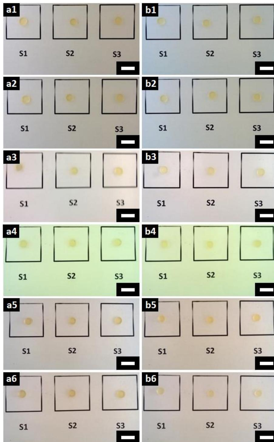
**Fig. S13:** Pictures of PGS (cured at 150 °C for 24 h) film samples during incubation in enzyme-free PBS solution ((a1): Day 0; (a2): Day 1; (a3): Day 7, (a4): Day 15; (a5): Day 23; (a6): Day: 31), and in PBS solution with the addition of lipase enzyme ((b1): Day 0; (b2): Day 1; (b3): Day 7, (b4): Day 15; (b5): Day 23; (b6): Day: 31) under dynamic conditions for up to 31 days at 37 °C (scale bar: 1 cm).
