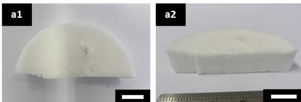
**Fig. S2:** (a1) Top and (a2) side view (cross section) of non-cured freeze-dried PLLA scaffold, produced with 2 g PLLA and 40 mL 1,4-dioxane (scale bar: 1cm).
