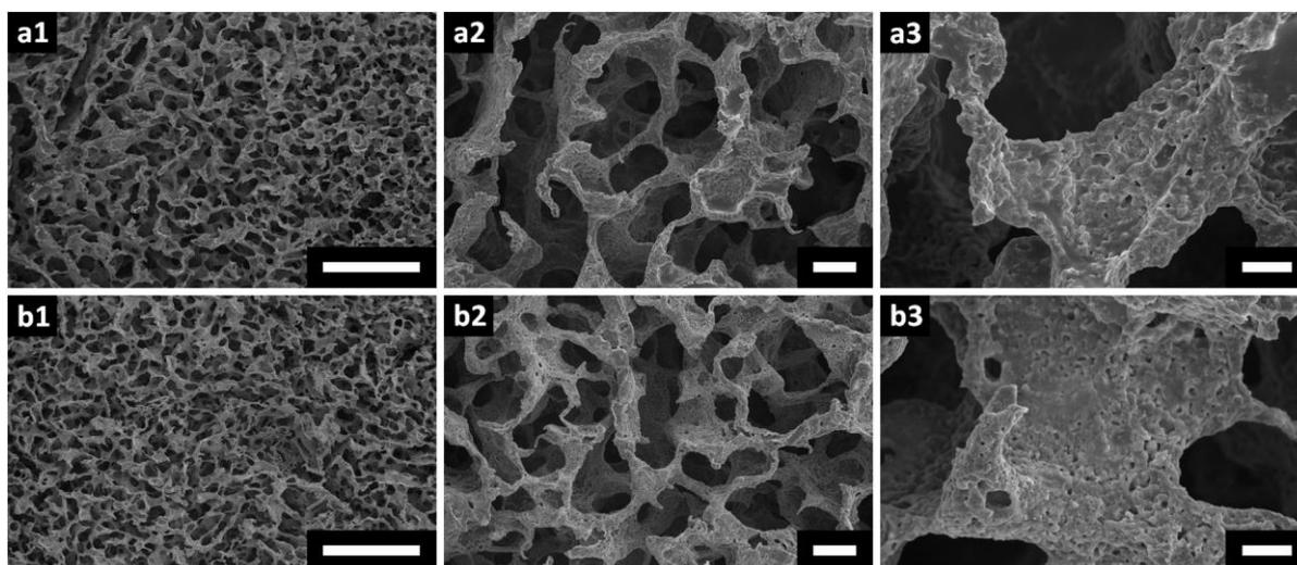
**Fig. S18:** SEM micrographs of PGS/PLLA scaffold specimens with a weight ratio of 2.5:1, after 31 days at 37 °C in (a1-3) enzyme-free PBS solution and (b1-3) in enzyme-containing PBS solution ((a1, b1) scale bar: 1 cm; (a2, b2) scale bar: 100  $\mu\text{m}$ ; (a3, b3) scale bar: 30  $\mu\text{m}$ ).
