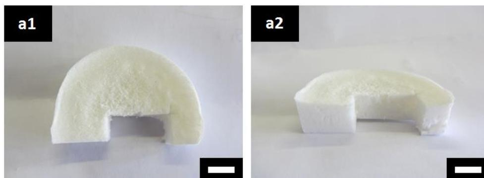
**Fig. S8:** (a1) Top and (a2) side view of cured PGS/PLLA blend scaffold with a weight ratios of 2.5:1 (scale bar: 1cm).
