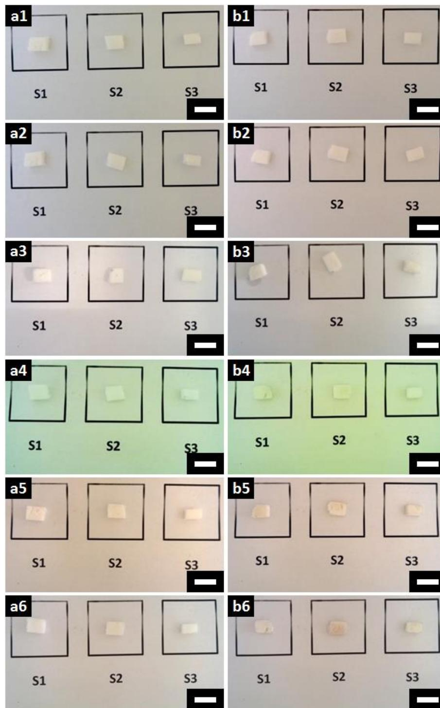
**Fig. S17:** Pictures of PGS/PLLA scaffold samples with a weight ratio of 2.5:1 during incubation in PBS solution ((a1): Day 0; (a2): Day 1; (a3): Day 7, (a4): Day 15; (a5): Day 23; (a6): Day: 31), and in PBS solution with the addition of lipase enzyme ((b1): Day 0; (b2): Day 1; (b3): Day 7, (b4): Day 15; (b5): Day 23; (b6): Day: 31) under dynamic conditions for up to 31 days at 37 °C (scale bar: 1 cm).
