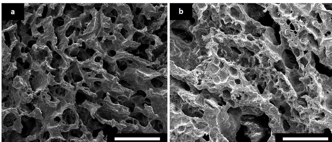
**Fig. S7:** SEM micrographs of cured PGS/PLLA blend scaffolds with a weight ratios of (a) 3.5:1, (b) 4:1 (scale bar: 500  $\mu\text{m}$ ).
