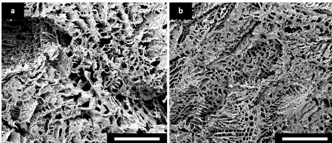
**Fig. S4:** SEM micrographs of cured PGS/PLLA blend scaffolds with a weight ratios of (a) 2:2, (b) 2:3 (scale bar: 500  $\mu\text{m}$ ).
