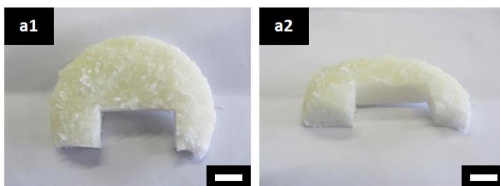
**Fig. S11:** (a1) Top and (a2) side view of cured PGS/PLLA blend scaffold with a weight ratio of 4:1 (scale bar: 1cm).
