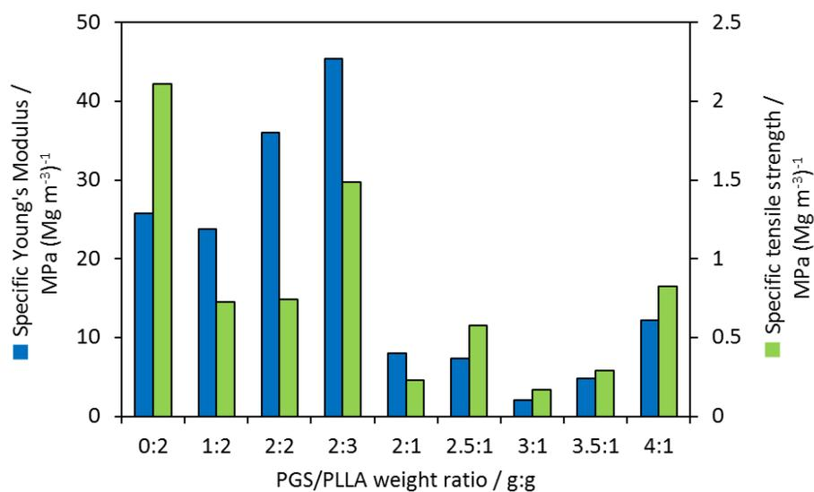
**Fig. S12:** Specific Young's modulus and specific tensile strength for PLLA and cured PGS/PLLA blend scaffolds with different weight ratios.
