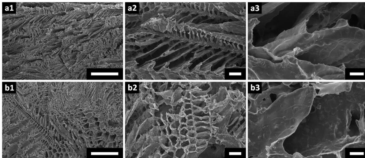
**Fig. S16:** SEM micrographs of PLLA scaffold specimens, after 31 days at 37 °C in (a1-3) enzyme-free PBS solution and (b1-3) in enzyme-containing PBS solution ((a1, b1) scale bar: 1 cm; (a2, b2) scale bar: 100  $\mu\text{m}$ ; (a3, b3) scale bar: 30  $\mu\text{m}$ ).
