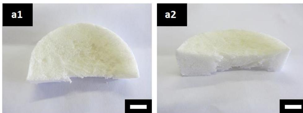
**Fig. S10:** (a1) Top and (a2) side view of cured PGS/PLLA blend scaffold with a weight ratio of 3.5:1 (scale bar: 1cm).
