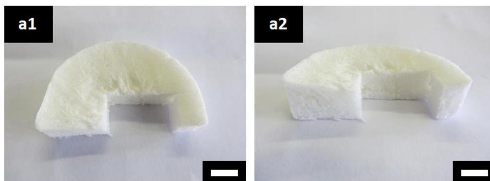
**Fig. S9:** (a1) Top and (a2) side view of cured PGS/PLLA blend scaffold with a weight ratios of 3:1 (scale bar: 1cm).
