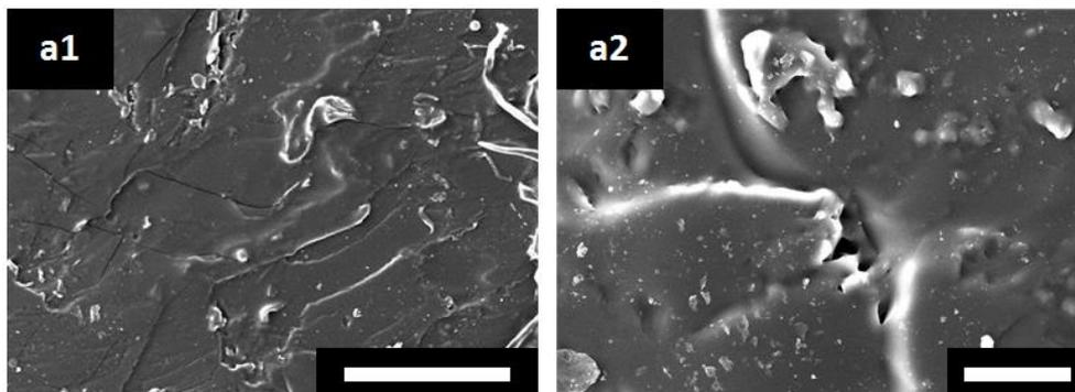
**Fig. S1:** (a1-2) SEM micrographs of the cured PGS film surface, after 24h ethanol extraction ((a1) scale bar: 200 $\mu$ m, (a2) scale bar: 50 $\mu$ m).
