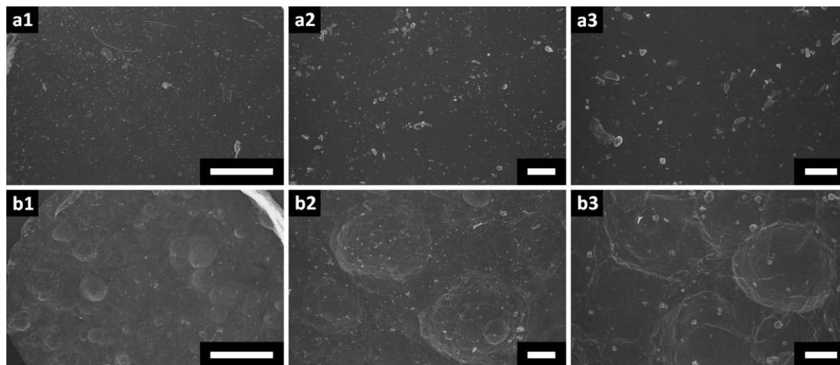
**Fig. S14:** SEM micrographs of PGS film (cured at 150 °C for 24 h) specimens with a weight ratio of 2.5:1, after 31 days at 37 °C in (a1-3) enzyme-free PBS solution and (b1-3) in enzyme-containing PBS solution ((a1, b1) scale bar: 1 cm; (a2, b2) scale bar: 100  $\mu\text{m}$ ; (a3, b3) scale bar: 30  $\mu\text{m}$ ).
