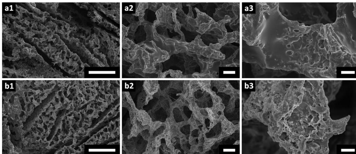
**Fig. S20:** SEM micrographs of PGS/PLLA scaffold specimens with a weight ratio of 2.5:1, after 31 days at 37 °C in (a1-3) enzyme-free PBS solution and (b1-3) in enzyme-containing PBS solution ((a1, b1) scale bar: 1 cm; (a2, b2) scale bar: 100 μm; (a3, b3) scale bar: 30 μm).
