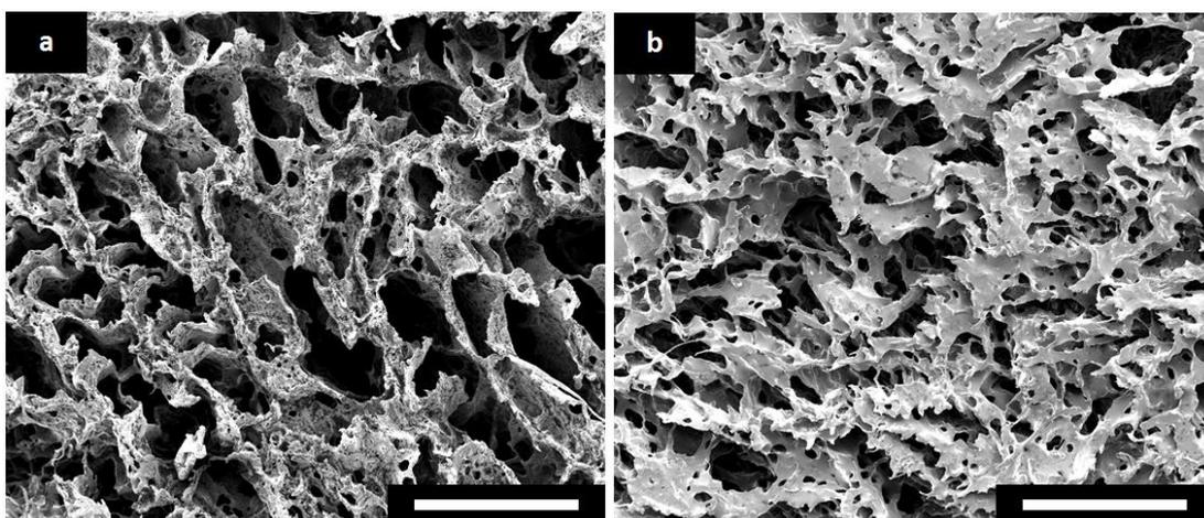
**Fig. S5:** SEM micrographs of cured PGS/PLLA blend scaffolds with a weight ratios of (a) 1:2, (b) 2:1 (scale bar: 500  $\mu\text{m}$ ).
