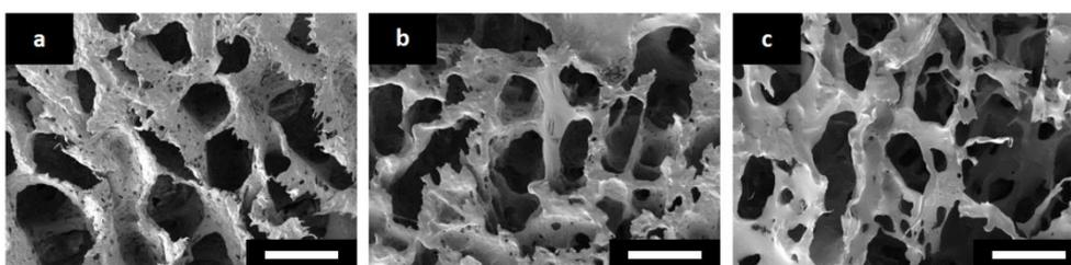
**Fig. S3:** SEM micrographs of pre-PGS/PLLA blend foams with a weight ratios of (a) 2:3, (b) 2:2 and (c) 2:1 (scale bar: 100 $\mu$ m).
