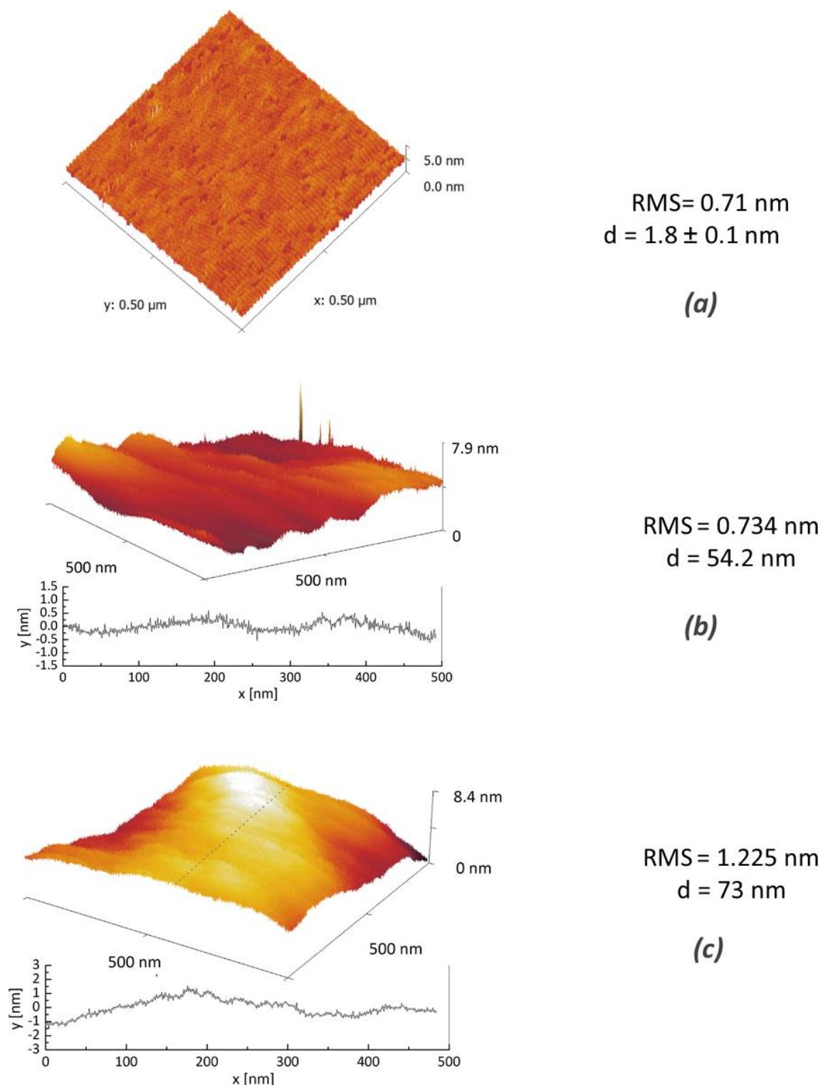
**Figure S2.** Tapping mode AFM images of functionalized silicon wafer substrates with: (a) CTA-1; (b) living PHEMA brushes ( $d = 54.2 \text{ nm}$ ); (c) chain extended PHEMA brushes ( $d = 73 \text{ nm}$ ). Chain extension was performed on a PHEMA functionalized substrate with initial  $d = 40.5 \text{ nm}$  (not shown). Thicknesses were measured by ellipsometry.
