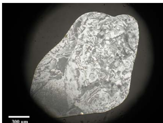
Photomicrograph of I-7 on a glass slide with a cover glass in) the SmC phase at 123.0 °C.
