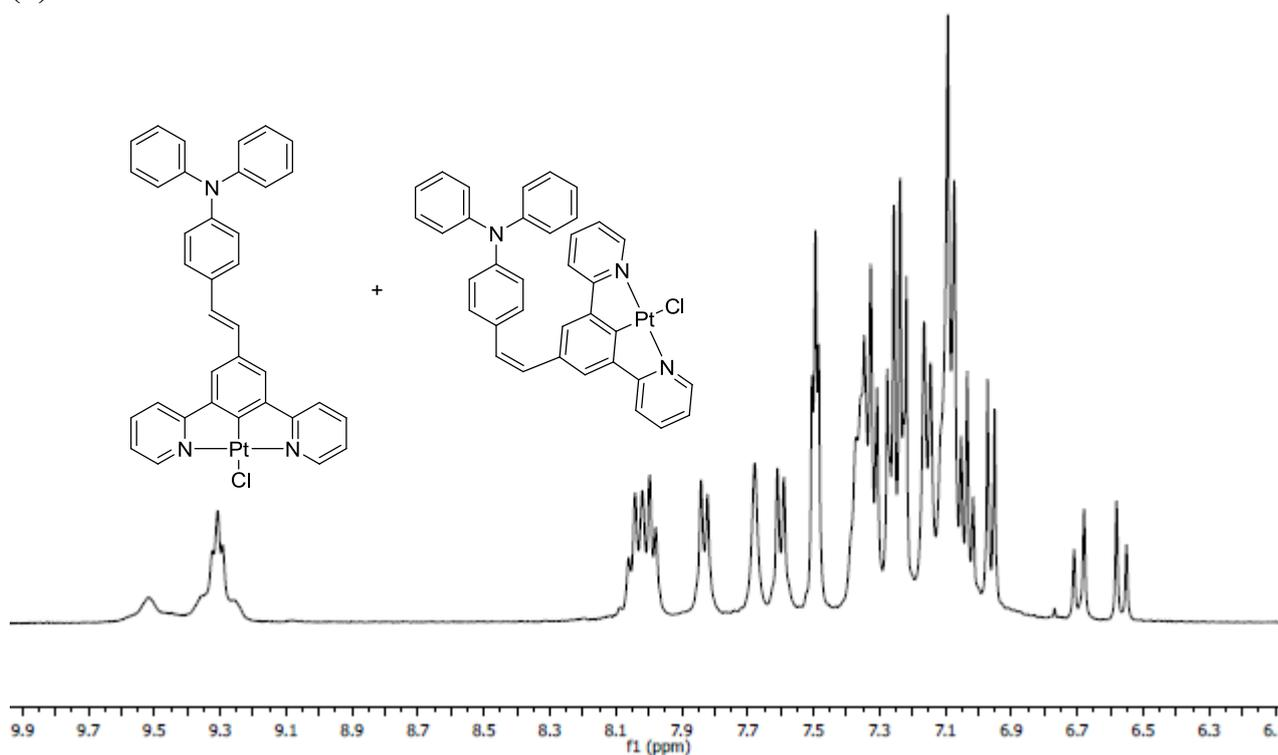
**Figure S1** <sup>1</sup>H NMR spectra (400 MHz) for PtL<sup>2</sup>Cl in CD<sub>2</sub>Cl<sub>2</sub>: (a) freshly prepared sample, (b) after exposure of the solution to solar light for 2 h.
