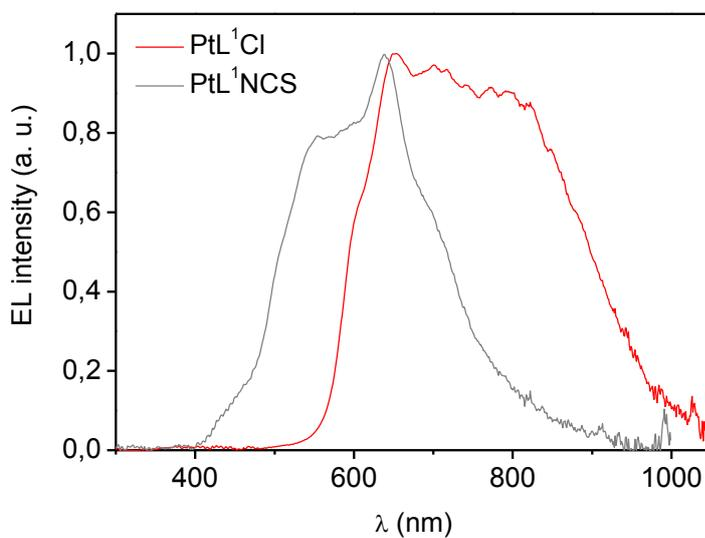
**Figure S5** Electroluminescence spectra of OLEDs based on PtL<sup>1</sup>Cl or PtL<sup>1</sup>NCS neat film as the emitting layer.
