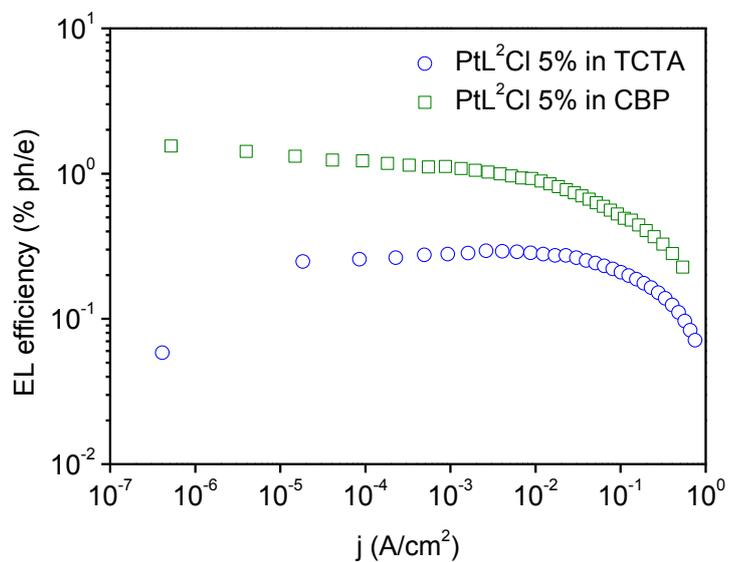
**Figure S7** External quantum efficiencies versus electric current density for the OLEDs based on PtL<sup>2</sup>Cl diluted in TCTA or CBP as emitting layer.
