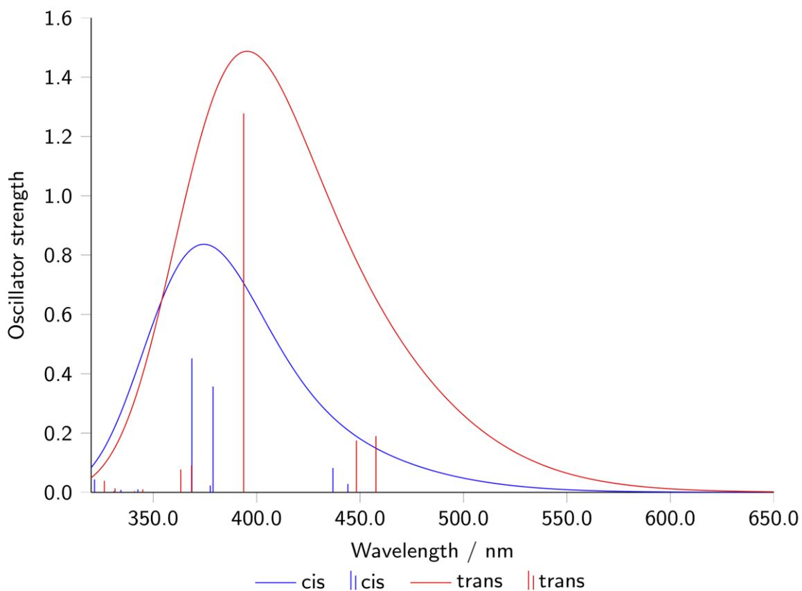
**Figure S3** Simulated absorption spectra in the near-UV region for the *trans* (red) and *cis* (blue) forms of PtL<sup>2</sup>Cl, convoluted from the individual calculated excitations represented by the vertical lines.
