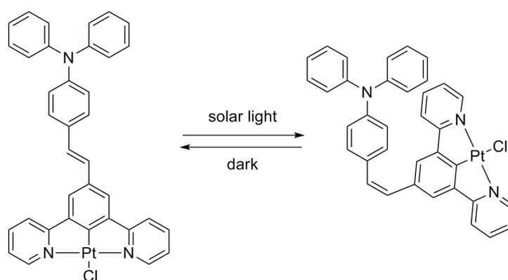
The  $^1\text{H}$  NMR spectrum in  $\text{CD}_2\text{Cl}_2$  of freshly prepared  $\text{PtL}^2\text{Cl}$  is shown in Figure 1(a), putting in evidence the presence of the *trans* isomer only. After 2 h under solar light exposure at room temperature in  $\text{CD}_2\text{Cl}_2$ , a mixture of *cis* and *trans* isomers is obtained {Figure 4(b)}. Simply leaving the solution in the dark for 18 h restores the *trans* isomer. No isomerisation is detectable in the solid state.
