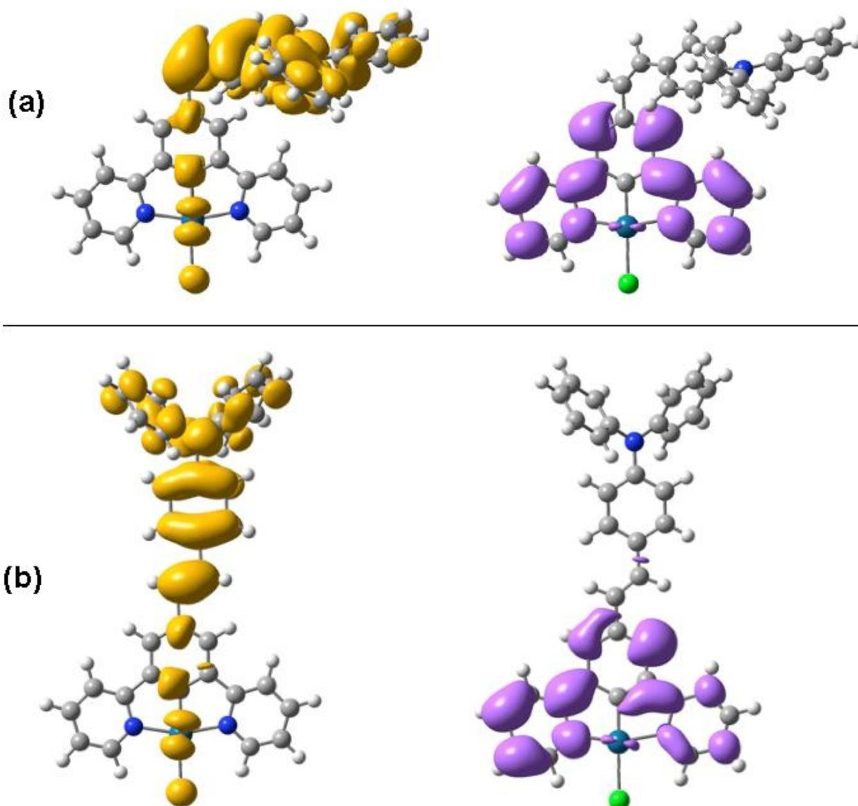
**Figure S4** Density difference plots for the lowest singlet excitations of the *cis* (a) and *trans* (b) forms of  $\text{PtL}^2\text{Cl}$  calculated at the ground state geometry, using PBE0 with the PCM model for  $\text{CH}_2\text{Cl}_2$ . Yellow and purple represent zones of depletion and augmentation of electron density in the first singlet excitation versus the  $S_0$  ground state.
