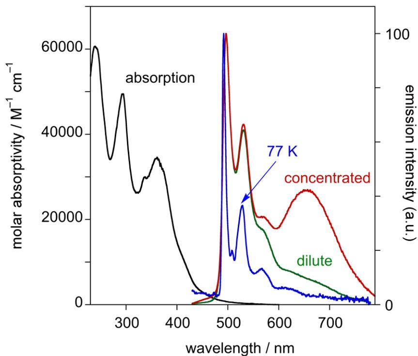
**Figure S2** Absorption spectrum of PtL<sup>1</sup>NCS in CH<sub>2</sub>Cl<sub>2</sub> at 298 K (black line); emission spectra under the same conditions for solutions of concentration  $1.24 \times 10^{-5}$  and  $1.03 \times 10^{-4}$  M (green and red lines respectively), and the emission spectrum at 77 K in a glass of diethyl ether / isopentane / ethanol (2:2:1 v/v) (blue line).
