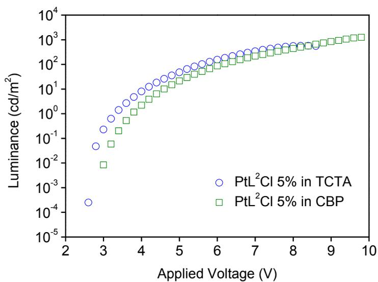
**Figure S6** Luminance versus applied voltage for OLEDs based on PtL<sup>2</sup>Cl diluted in TCTA or CBP as the emitting layer.
