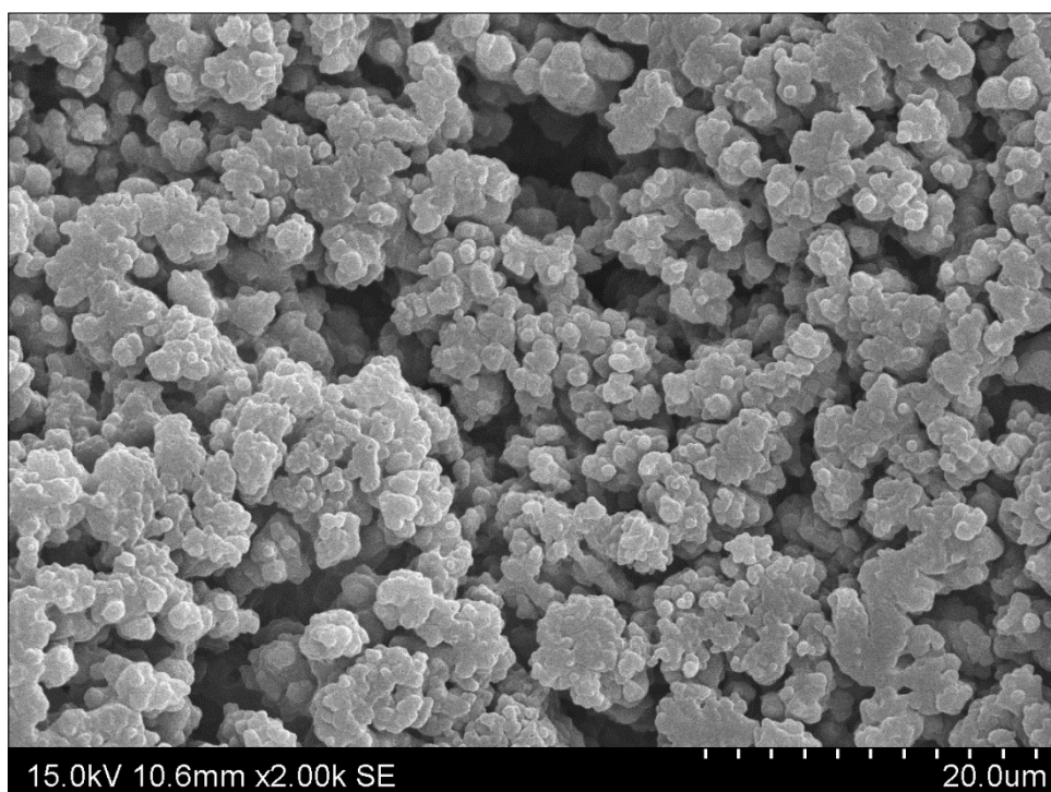
Figure S13: HF etched polynorbornene (PNBE) with 50 wt% TiO 2
