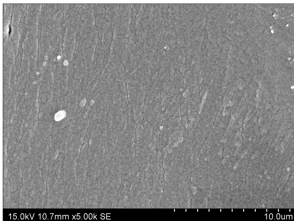
Figure S8: Poly((3aR,7aS)-2-butyl-3a,4,7,7a-tetrahydro-1H-4,7-epoxyisoindole-1,3(2H)-dione) poly( M1 ) with 10 wt% TiO 2 & AcAc
