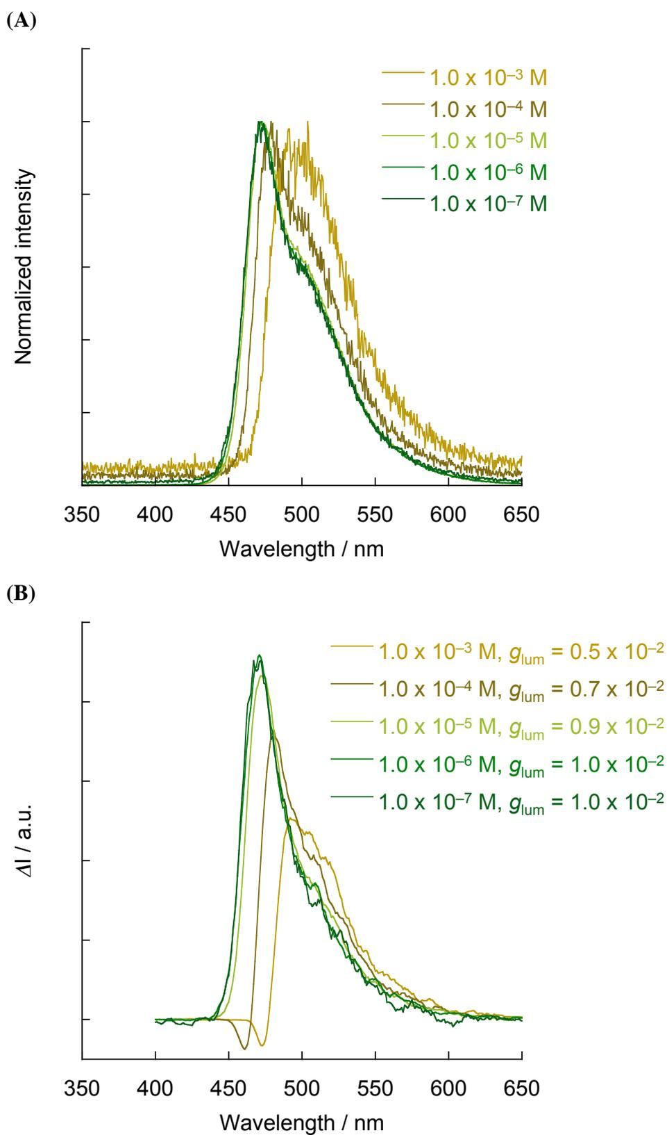
**Figure S27.** Concentration effect on (A) PL and (B) CPL spectra of (*R<sub>p</sub>*)-**5PhC** in  $\text{CHCl}_3$ , excited at 330 nm.
