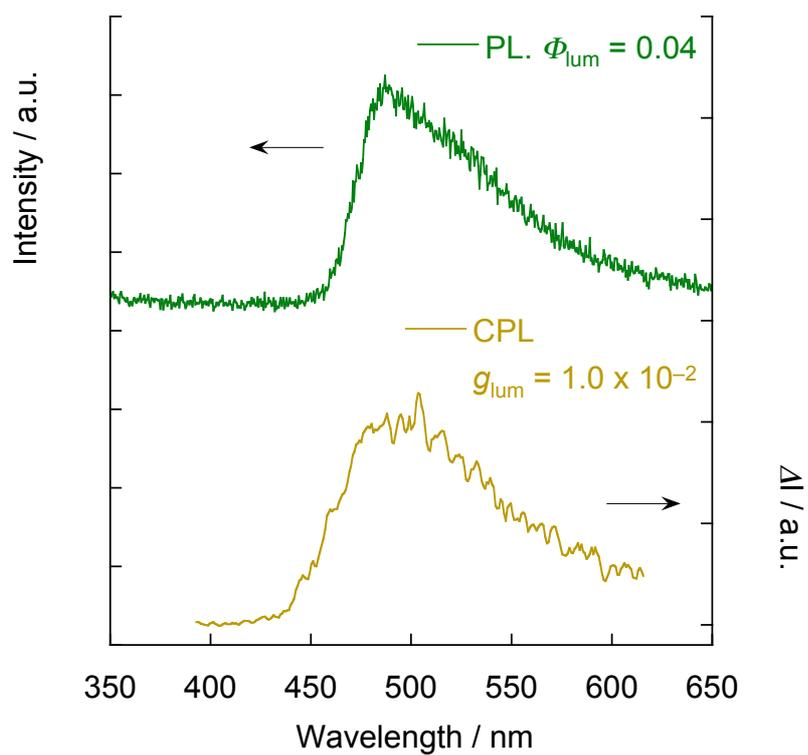
**Figure S28.** PL and CPL spectra of the (*R<sub>p</sub>*)-**5PhC** cast film from the CHCl<sub>3</sub> solution ( $1.0 \times 10^{-3}$  M), excited at 333 nm.
