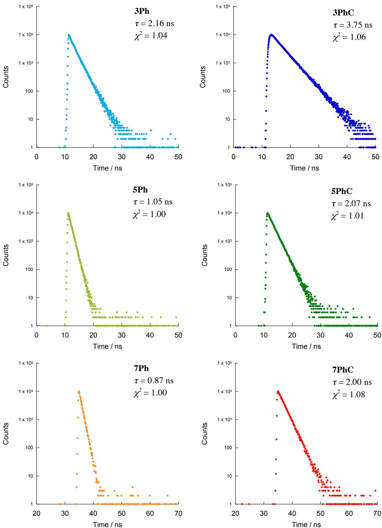
**Figure S23.** PL lifetime decay curves of  $(R_p)$ -isomers in  $\text{CHCl}_3$  ( $1.0 \times 10^{-6}$  M) at room temperature, excited at 375 nm with LED laser. Their PL peak tops were monitored.  $(S_p)$ -Isomers exhibited identical profiles.
