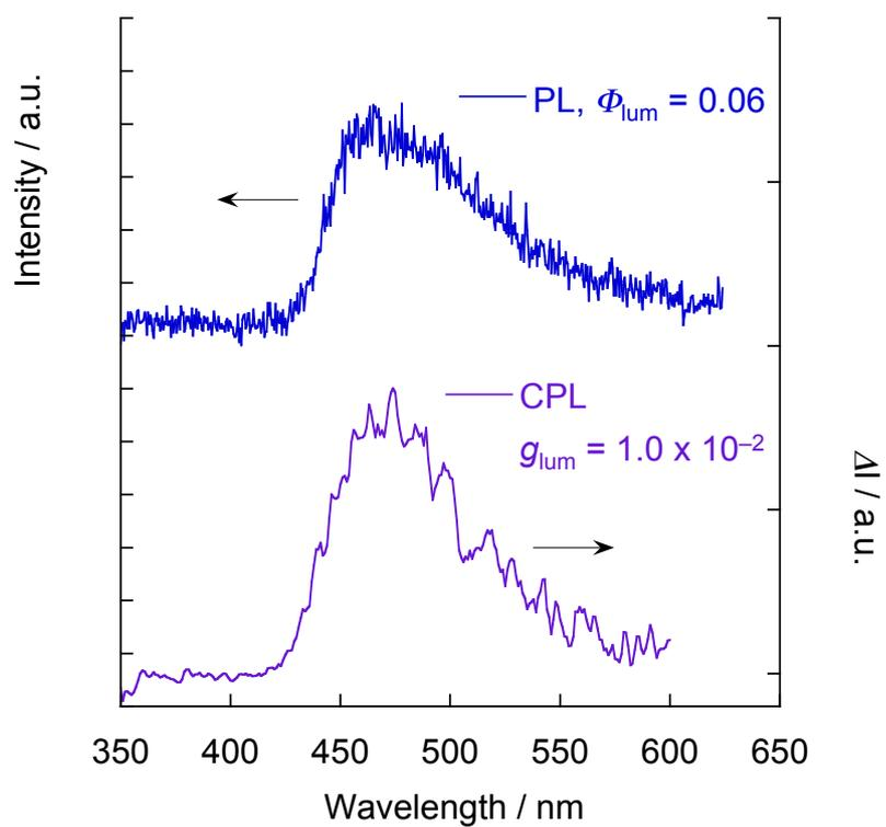
**Figure S26.** PL and CPL spectra of the (*R<sub>p</sub>*)-**3PhC** cast film from the CHCl<sub>3</sub> solution ( $1.0 \times 10^{-3}$  M), excited at 316 nm.
