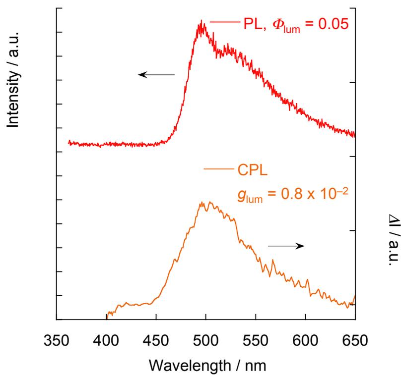
**Figure S30.** PL and CPL spectra of the (*R<sub>p</sub>*)-**7PhC** cast film from the CHCl<sub>3</sub> solution ( $1.0 \times 10^{-3}$  M), excited at 333 nm, excited at 352 nm.
