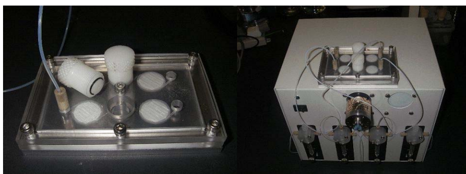
Figures 1 Fabricated two-lanes membrane device (left) and flow system (right).
