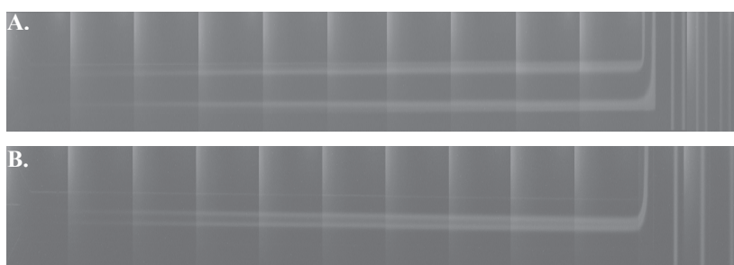
Figure 4. Micrographs of bioluminescence in straight channel of microfluidic device with different infusion methods: ATP solution in the middle (A), reagent solution in the middle (B). ATP solution ( 10^{-3} M) occupied 70% of total 8 \mu\text{l}/\text{min} of flow.
