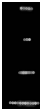
Figure 2. One-dimensional aggregation of 10 \mu\text{m} beads in four subsequent pressure nodes.
