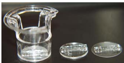
Figure 4. PDMS chips bonded to (from left to right) a porous membrane, a PDMS plate, and a glass plate (12 mm diameter).
