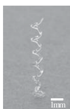
Fig. 6 A micro-coil spring. L.D.: 0.2mm, O.D.: 0.9mm, Pitch: 0.8mm, N=5, Fabrication time: 3min. Material: PLGA.
