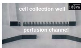
Figure 3 (left) Scanning electron micrograph of devices before assembly. Due to the high aspect ratios (1:10 to 1:20), the posts are fragile and can break off or stick to each other during handling.
