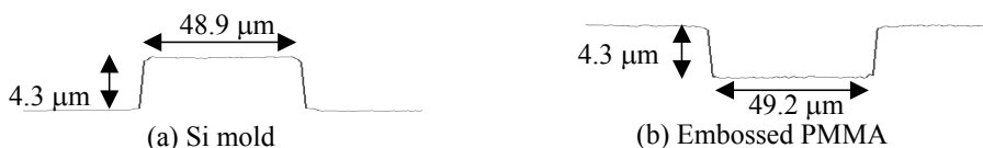
Figure 3. Cross sectional profile of the dam at the mold (a) and the embossed plate (b).
