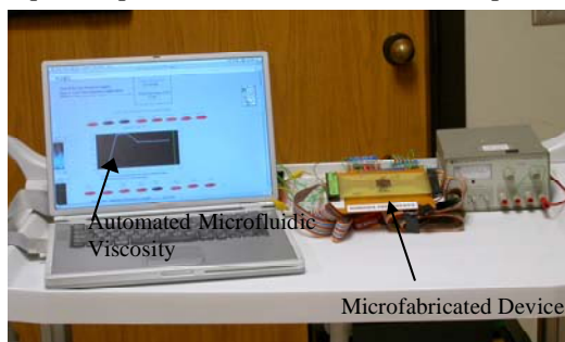
Fig.3: Automated and Portable Viscosity Measurement System. The setup consists of a microfluidic device with digital electrode sensors, external electronics, data acquisition accessories and a laptop computer.
