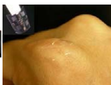
Fig. 3 The needles array fabricated on a flexible membrane substrate for compliant applications has been successfully realized in this study. The substrate employed here was PDMS.
