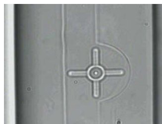
Figure 4 A microrotor with an outer casing fabricated inside a microchannel
