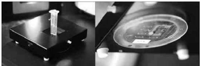
Figure 1. Portable Setup: Images of (left) top view of the portable desktop iDEP unit with power supply and (right) underside showing the iDEP polymer device containing 8 separate channels.
