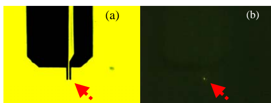
Fig. 6. The observation of tip of tweezer-type AFM probe. (a) bright field and (b) fluorescence field. Fluorescence of chromosome fragment could be observed at the tip of the tweezer-type probe.
