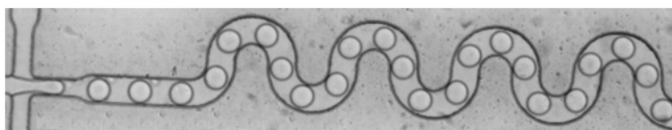
Figure 2. Droplets of methanol being formed at a flow-focusing junction in fluorinated oil with 1 mM fluorinated surfactant molecule X.
