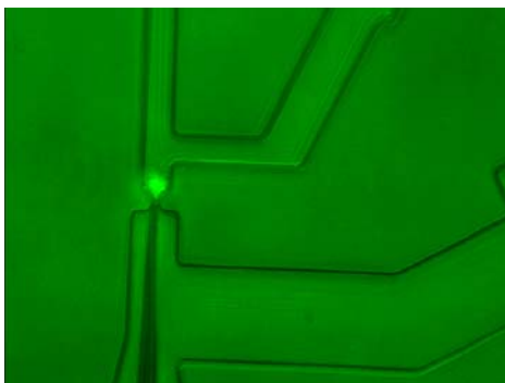
Figure 3: Injection area with a cell dyed with Acridine Orange (vital dye) for visualization purposes
