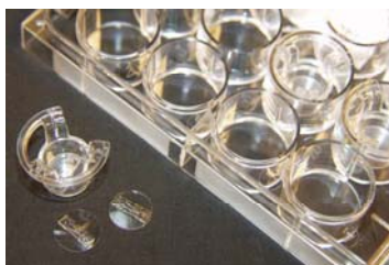
Figure 5. The cell culture devices are compatible with a multi-wellplate format.
