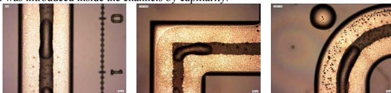
Figure 4. Images of microchannels of different geometries after UV grafting.
