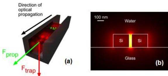
Figure 1. Slot Waveguide-Integrated Optofluidic Trapping Architecture (IOTA) (a) Schematic showing trapping of nanoparticles in exposed-mode slot region between two silicon waveguides. (b) Cross-sectional optical field distribution of slot waveguide submerged in water ( $n = 1.33$ ).
