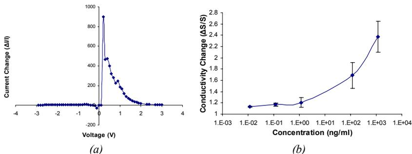
Figure 5. (a) Characterization of  $V_{ds}$  for maximum output and (b) conductivity change of photovoltaic polymer coated SWNT according to the concentration of cTnT
