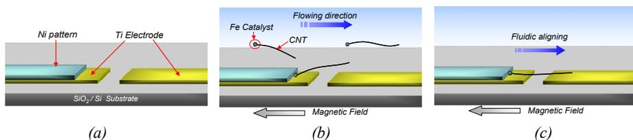
Figure 2: Microfluidic self-assembly procedure of CNT. (a) Self-aligned Ni pattern on Ti electrode fabricated by CUM, (b) Magnetic capturing Fe catalyst at the end of SWNT and (c) Fluidic alignment of CNT parallel to flow direction.
