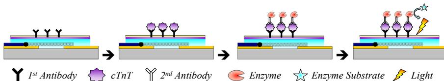
Figure 4. Sequences for on-chip chemiluminescent immunoassay with CNT photodetector
