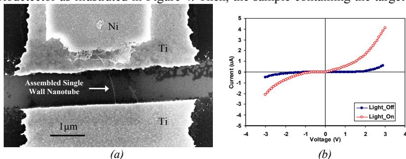
Figure 3. Assembled SWNT: (a) SEM image and (b) I-V curve under the incident light
