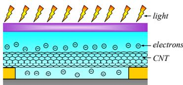
(b) Charge generation in photovoltaic polymer under light irradiation
