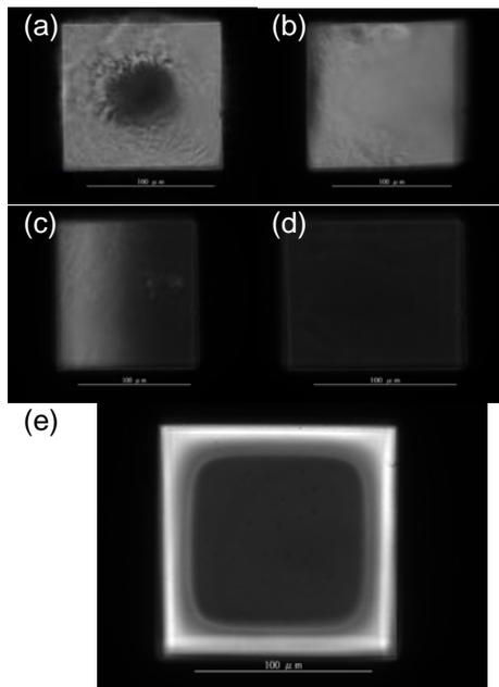
Figure 2. BLM formation. (a) Bottom droplet at the aperture. (b)-(d) Top droplet passing the aperture. (e) BLM formed.
