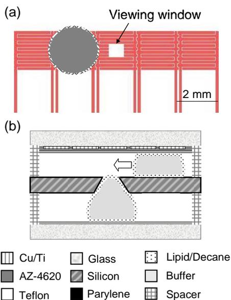
Figure 1. BLM formation device configuration. (a) Top view of interdigitated electrowetting electrode design for encapsulated droplet actuations. (b) Cross-section of the device containing three parallel plates.
