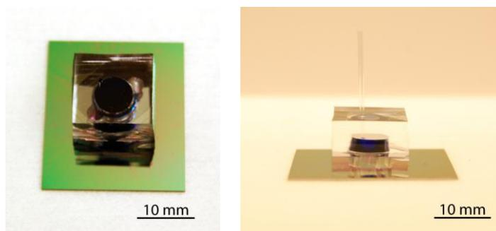
Figure 2. Side and top view of the prototype micro-dispenser.
