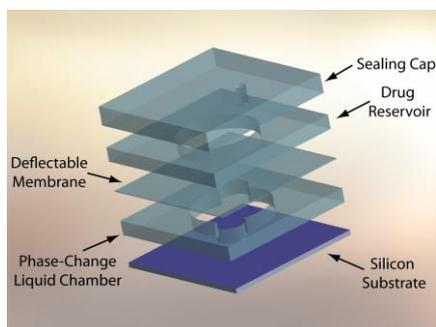
Figure 1. 3D Exploded sketch of the micro-dispenser.
