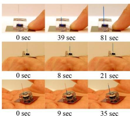
Figure 3. Time frame images of the device, pumping when in direct contact with the skin.
