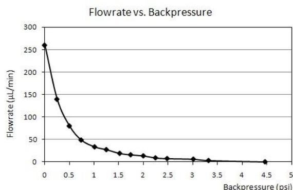
Figure 5. Flowrate vs. backpressure for FC-3284 phase change liquid.
