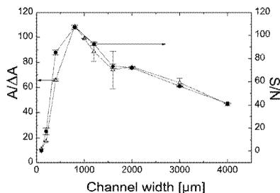
Figure 4: Verification of the relation  $S/N \approx A/\Delta A$  (open symbols:  $A/\Delta A$ , filled symbols:  $S/N$ ).
