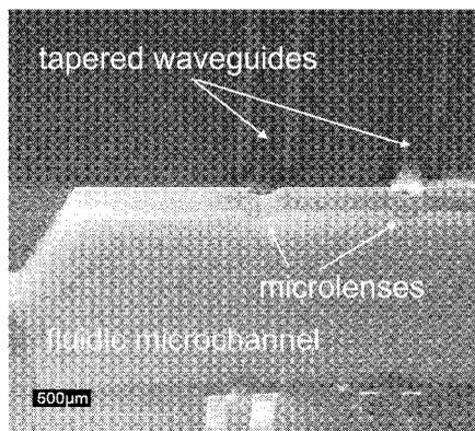
Figure 1: SEM picture of a microstructure for S/N measurements fabricated by structuring a single SU-8 layer.
