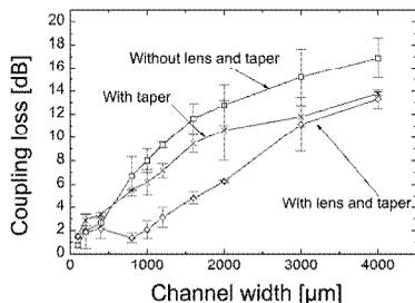
Figure 3: Coupling loss as a function of optical path length for different configurations of beam shaping components (the connecting lines are for guidance only).
