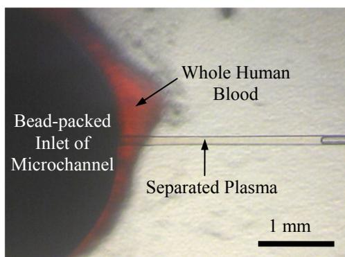
(a) Separated plasma from whole blood at the bead-packed inlet of microchannel
