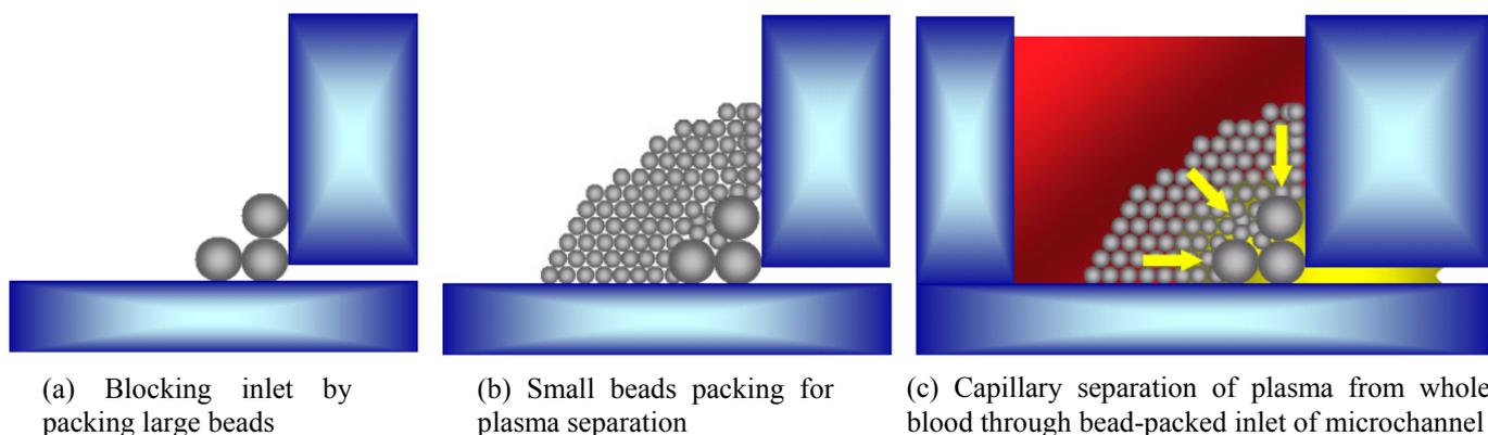
Figure 1. Schematic illustrations of hetero-packed beads and blood/plasma separation.
