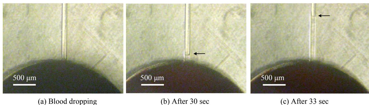
Figure 3. Rapid separation of plasma by the bead-packed inlet of microchannel (500  $\mu\text{m}$  scale bar).
