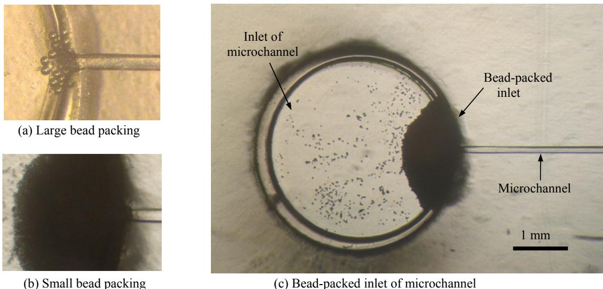
Figure 2. Microscopic picture of bead-packed inlet of microchannel for plasma extraction from whole blood.
