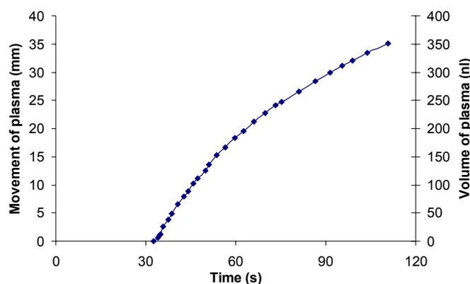
(b) Movement of separated plasma according to time
