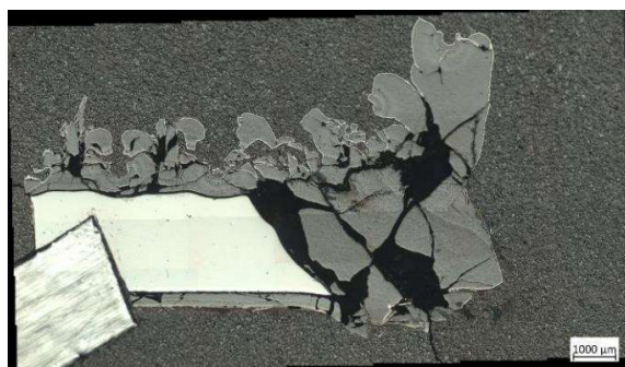
Figure 1: Optical micrograph of a finned 9Cr-1Mo steel sample after 15,000 hours of CO 2 exposure. After breakaway of the fins, oxidation degradation of the tube wall is in a state of arrest.
