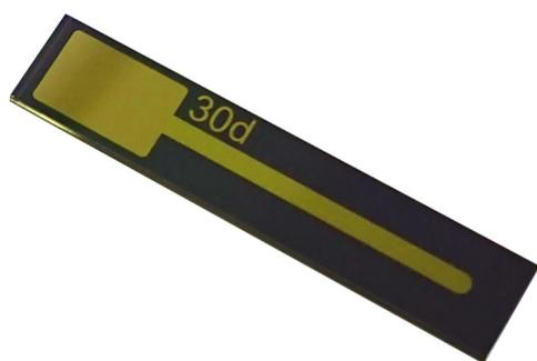
**Fig. 1** Microfabricated gold electrode, with a 30  $\mu\text{m}$  microdisc.
