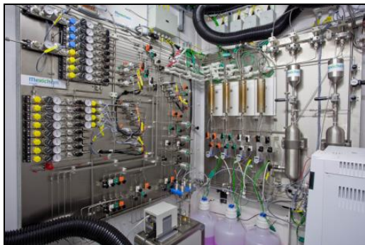
Figure 2. High-throughput atmospheric catalyst screening rig for hydrofluorination chemistry.
