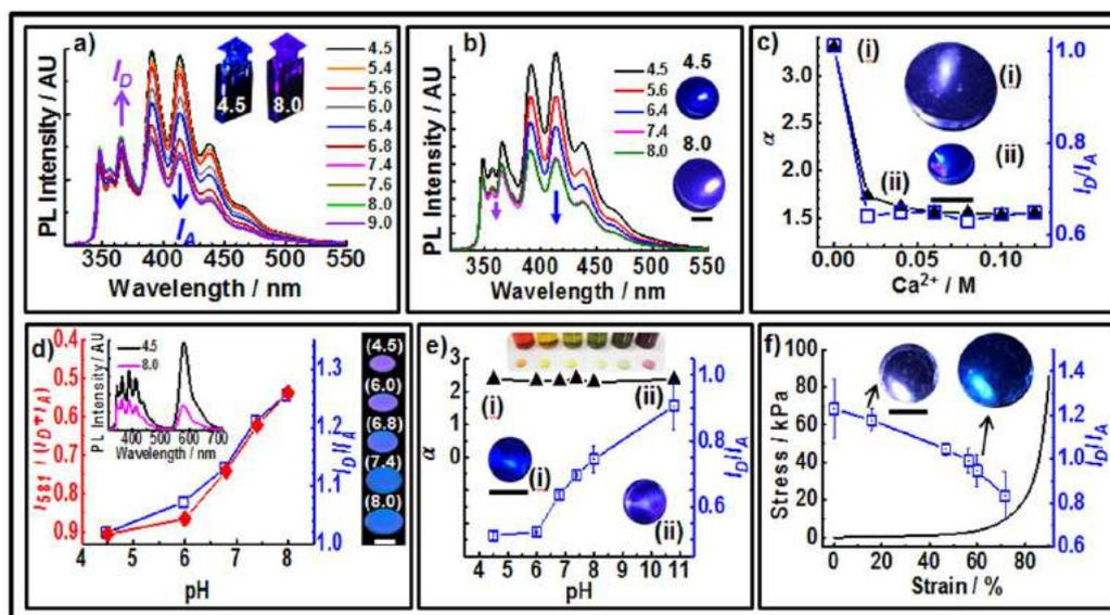
**Figure 1** PL of pH-responsive swelling NG<sub>Ph/An</sub> nanogel probe (a), DX NG(NG<sub>Ph/An</sub>) gels (b). Ca<sup>2+</sup>-triggered collapsed in DX NG(NG<sub>Ph/An</sub>) gels (c). Molecules monitored in DX NG(NG<sub>Ph/An</sub>) gels (d). pH-sensing PAAm-MBAAm(NG<sub>Ph/An</sub>) gel (e). Compressive-strain sensing in PAAm-Lap(NG<sub>Ph/An</sub>) gels (f).
