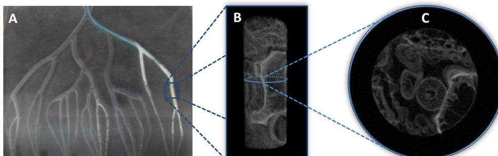
**Figure 1** – (A) Embolized channel of Vascular Flow Model. (B) Reconstructed microCT surface view. (C) Reconstructed 2D microCT cross section.
