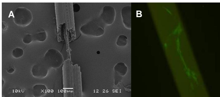
Figure 1: A) Scanning Electron Microscopy image of micro-HFs, showing the inner polycaprolactone and outer polystyrene, with the linear indents running parallel along the fibre. B) Live dead stain 6 days post-seeding of OECs and NG108s seeded at 20,000:1,000 cells/cm<sup>2</sup> respectively. Fibre was coated with Laminin.
