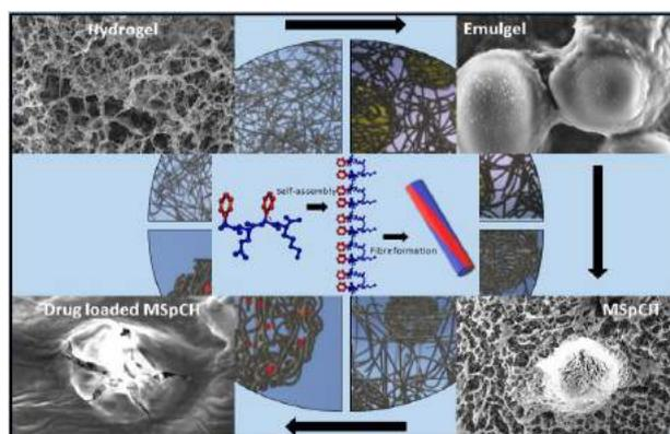
Figure 1: An illustration of the self-assembly of the amphiphilic ultra-short peptide and the versatile systems fabricated from the nanofibers
