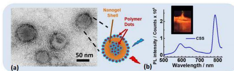
Figure 1: (a) Representative STEM image of CSS particles. Inset shows structure of the particles. (b) PL emission spectrum, and photograph (Inset), of CSS dispersion.
