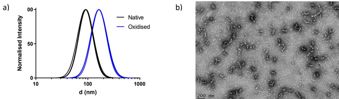
Figure 1: pHEA<sub>35</sub>-*b*-p(NIPAM-*st*-BAPE)<sub>250</sub> nanogel with a crosslinker to mCTA ratio of 5:1 a) DLS of the polymer at 0.1 wt% before and after oxidation of 37 °C, b) TEM prepared at room temperature of the nanogel at 0.05 wt%
