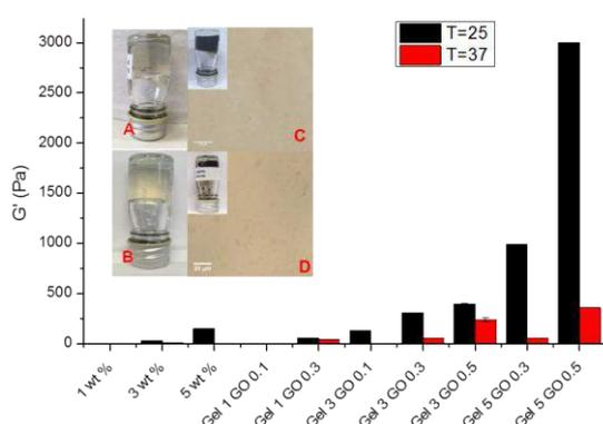
GO improves  $G'$  at 25 and 37°C which can be seen in Figure 1. This is due to favourable intermolecular interactions between GO sheets and gelatin fibres.
