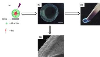
Figure 1: (a) Diffusion-driven co-assembly of G-actin and PA, (b) optical image of hydrogel formed, (c) hydrogel can be handled with a pair of tweezers, and (d) SEM image of PA-actin gel.
