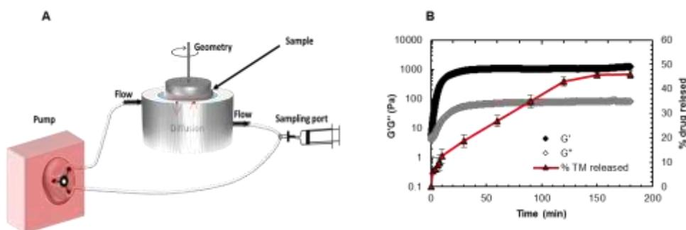
Figure 1: (A) Schematic diagram of the experimental set up of rheo-dissolution cell (B) Rheo-dissolution experiments of *in situ* gel forming ophthalmic formulation
