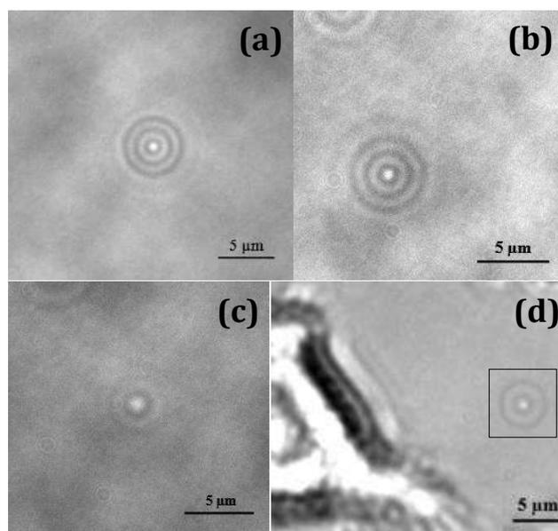
**Figure 1:** Photograph of the caustic in deionised water generated by: (a) 50 nm gold nanoparticle; (b) 50 nm BSA nanoparticle; (c) BSA protein. (d) 50 nm gold nanoparticle approaching the extracellular membrane of a fibroblast. Cell is out of focus to allow the correct formation of the particle caustic.
