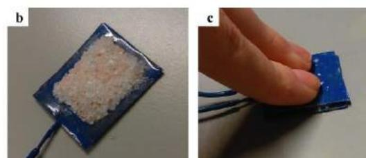
**FIGURE 1:** Generating voltage from amino acid crystals
