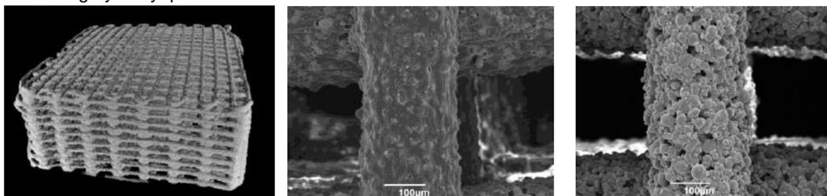
Figure 1: Left) micro CT image of a 3D printed composite scaffold. Middle, Right) SEM images of composite scaffolds with 60%wt and 84%wt hydroxyapatite, respectively.
