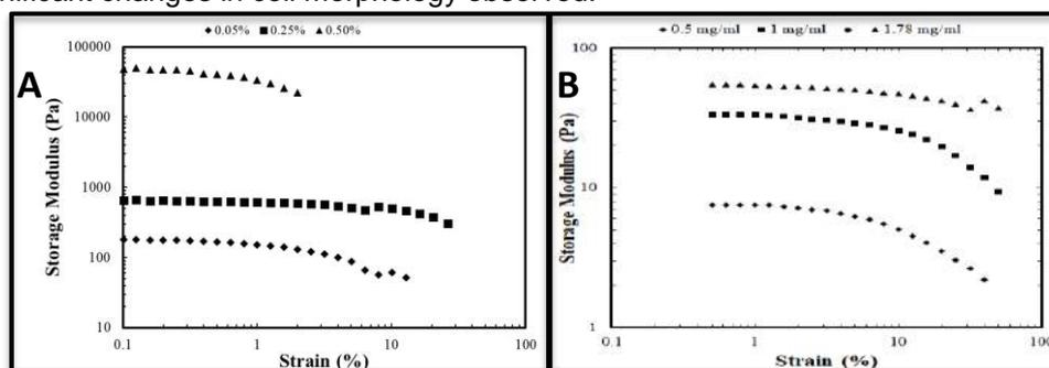
Figure 1: Strain amplitude sweep of tuneable synthetic (A) and collagen-based (B) hydrogels.
