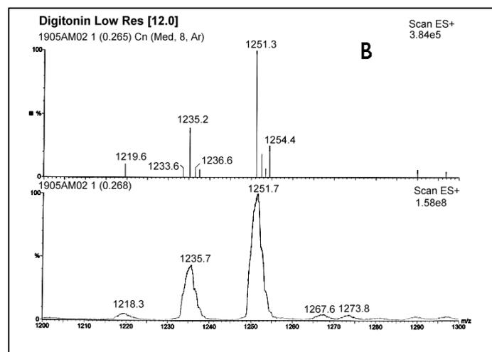
Figure 6b: Instrument incorrectly tuned
