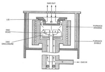
Samples and reference materials in pans sit on plates, which are in thermal contact with thermocouples. These are enclosed by a furnace, which enables heating/cooling of both. The heating/cooling can be controlled via a third thermocouple or the thermocouple of the reference material.
