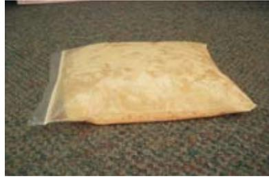
*Photograph showing the inflated bag of Sample C after 20 minutes*
