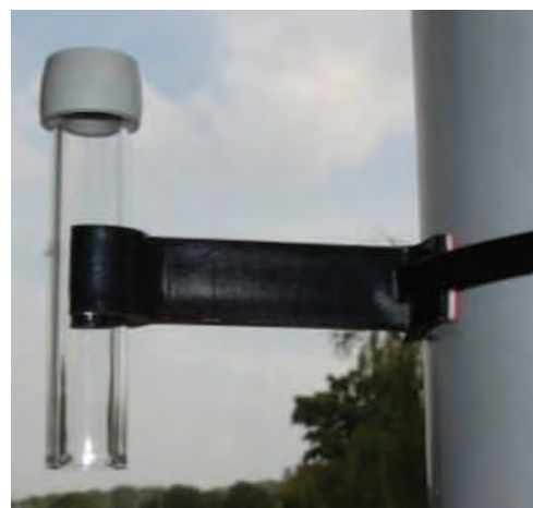
Figure 1: Schematic of a Palmes-type passive diffusion tube, and an example deployment (photo from Gradko International Ltd.).
