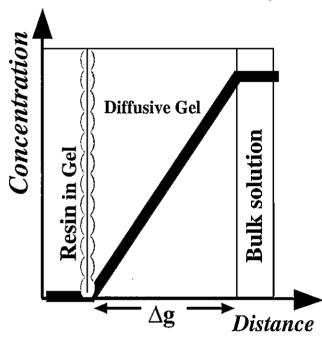
selective binding resin after passage through an open-pore gel. The simple plastic assembly can be deployed in situ in rivers and effluents where it automatically separates metal ions from solution. Metals are subsequently analysed conveniently and accurately in the laboratory. DGT has been important technique for the work described in this
