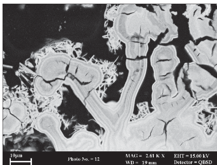
Figure 1 BSEM image showing detail of arsenic-rich iron oxyhydroxide cement coating the surfaces of altered waste fragments. It shows banded colloform oxyhydroxide gel material displaying shrinkage (desiccation) cracks. This is encrusted by more crystalline acicular oxyhydroxide.
