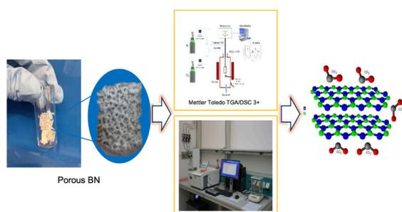
Figure 4. Schematic representation of CO<sub>2</sub> capture using porous boron nitride as an adsorbent.
