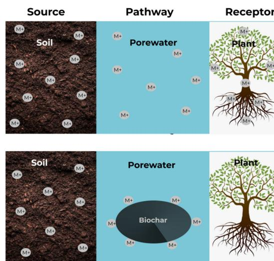
**Figure 3.** Conceptual model showing remediation of contaminant using biochar to break the source-pathway-receptor linkage
