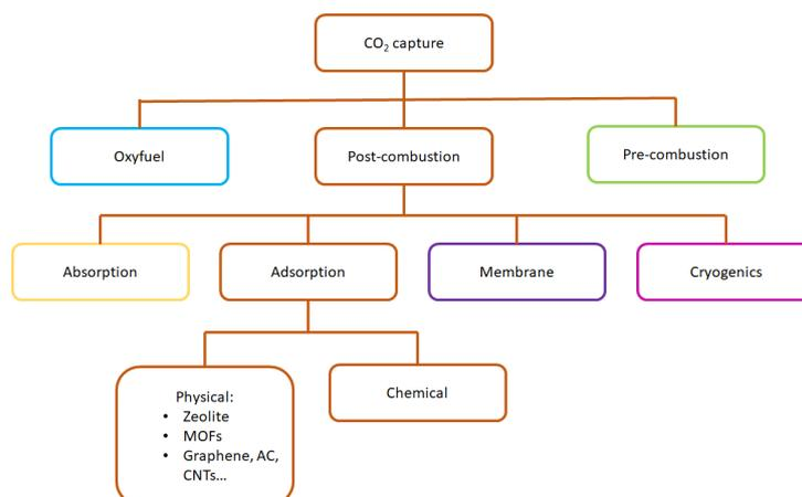
Figure 3. Different techniques of CO<sub>2</sub> capture [6].
