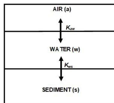
Figure 3. Illustration of a simple 3-compartment Level 1 model.
