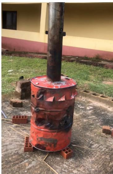
**Figure 2.** Picture of a pyrolysis kiln, locally made in Nigeria, from an oil barrel.
