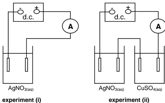
The circuits of two electrolysis experiments, (i) and (ii), are shown in the diagram. The electrodes were platinum and the ammeter reading was 0.5 A in both experiments.
