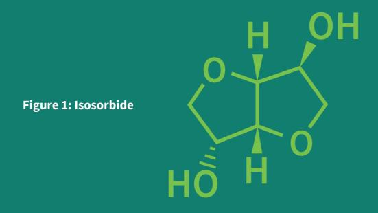
Researchers at the Korea Research Institute of Chemical Technology demonstrated that transparent polycarbonate sheets made with isosorbide outperform those made with the traditional, fossil fuel based, bisphenol A molecule in strength tests.<sup>7</sup>
